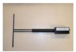
Figure 1 - Satimo COMOSAR Validation Dipole
