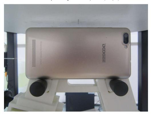
10mm body-worn Top Side Setup Photo (hotspot)
