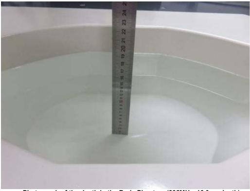
Photograph of the depth in the Body Phantom (835MHz, 16.0cm depth)
