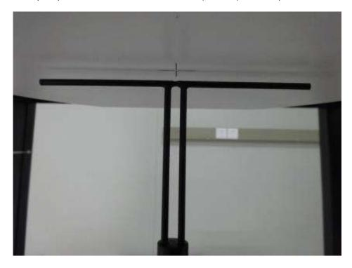
Photo of Dipole Setup
