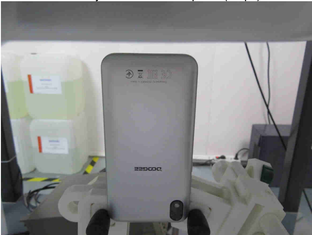
10mm body-worn Bottom Side Setup Photo (hotspot)
