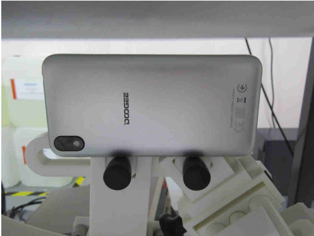
10mm body-worn Left Side Setup Photo(hotspot)
