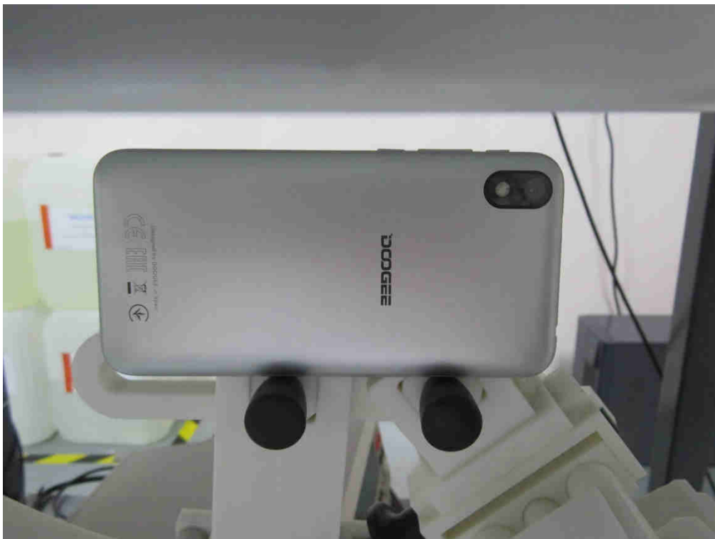
10mm body-worn Right Side Setup Photo (hotspot)
