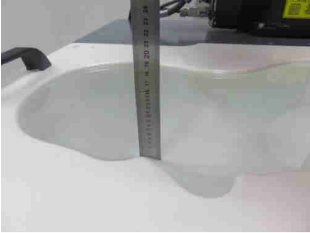
Photograph of the depth in the Head Phantom (2450MHz, 15.7cm depth)
