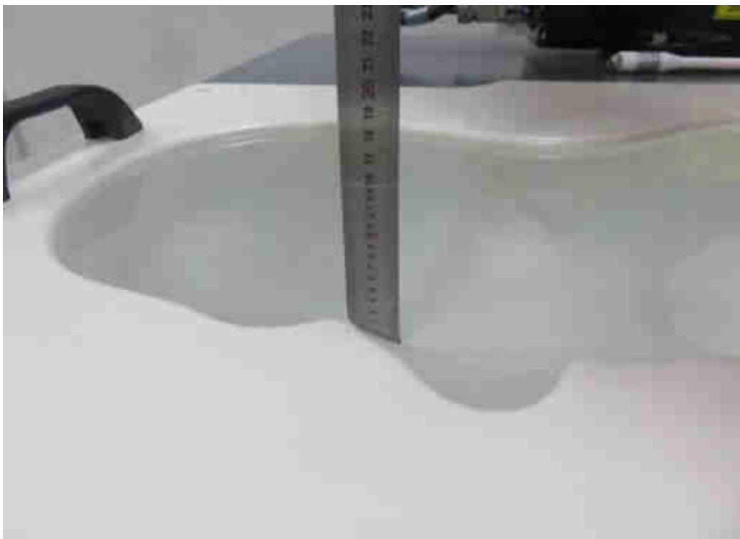
Photograph of the depth in the Head Phantom (1900MHz, 15.8cm depth)
