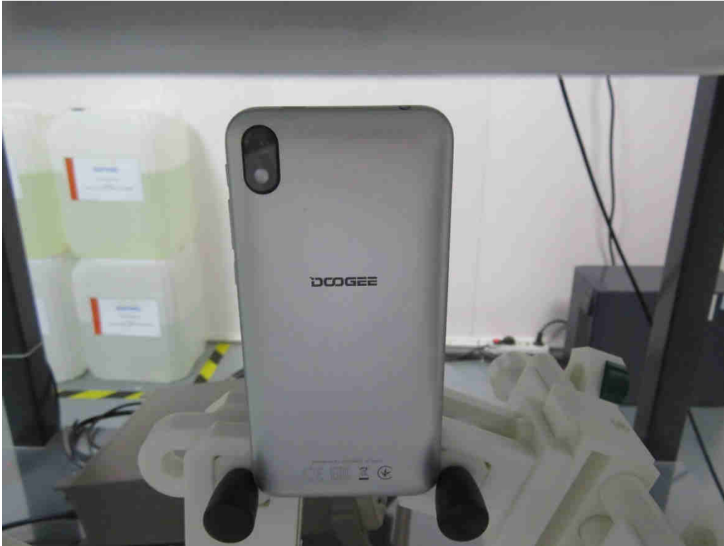
10mm body-worn Top Side Setup Photo (hotspot)
