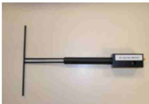
Figure 1 – Satimo COMOSAR Validation Dipole
