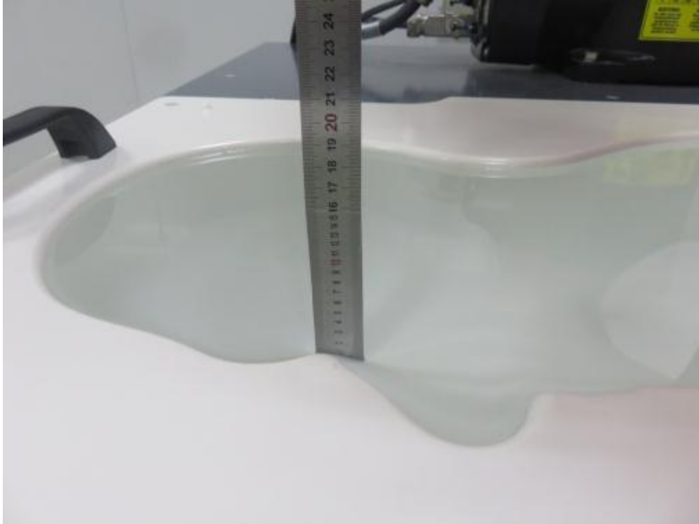
Photograph of the depth in the Head Phantom (2450MHz, 15.8cm depth)
