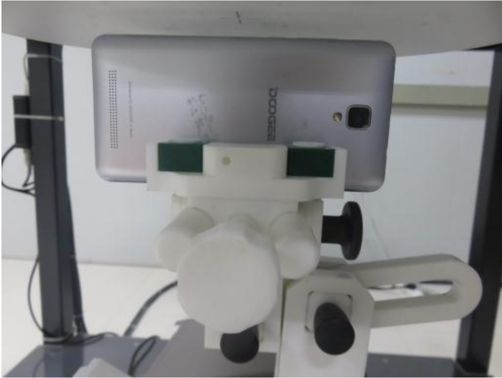
10mm body-worn Right Side Setup Photo(hotspot)
