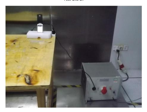
**Photograph - Spurious Emissions Radiated Test Setup**
