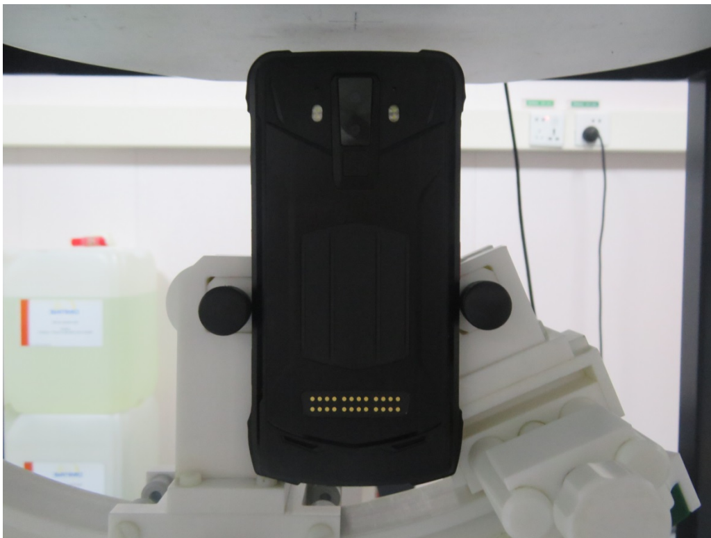
10mm body-worn Top Side Setup Photo (hotspot)
