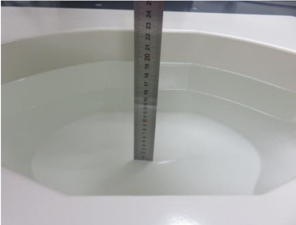
Photograph of the depth in the Body Phantom (1800MHz, 15.2cm depth)
