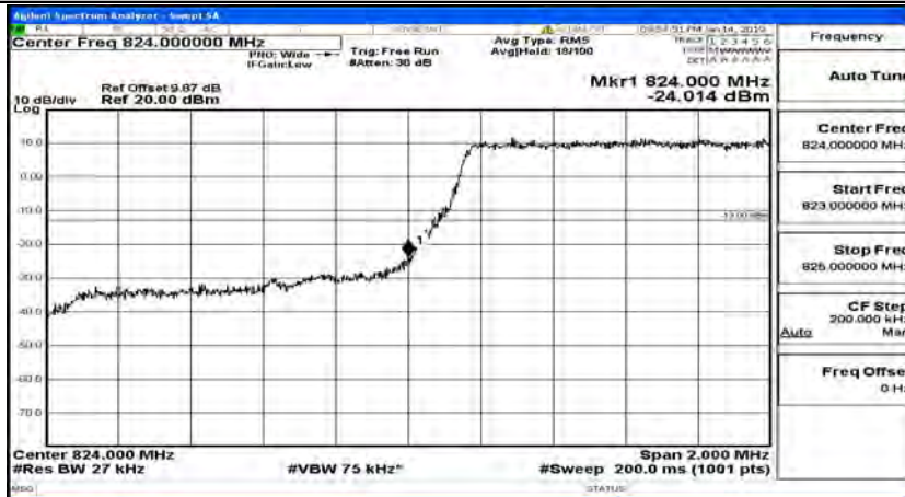
Band Edge Test Graph(s) (Channel Bandwidth: 1.4 MHz)_LCH_QPSK
