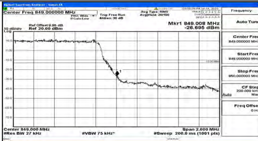
Band Edge Test Graph(s) (Channel Bandwidth: 1.4 MHz)_HCH_QPSK
