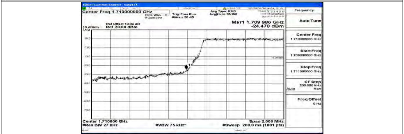
Band Edge Test Graph(s) (Channel Bandwidth: 1.4 MHz)_LCH_QPSK
