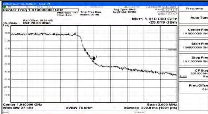
Band Edge Test Graph(s) (Channel Bandwidth: 1.4 MHz)_HCH_QPSK
