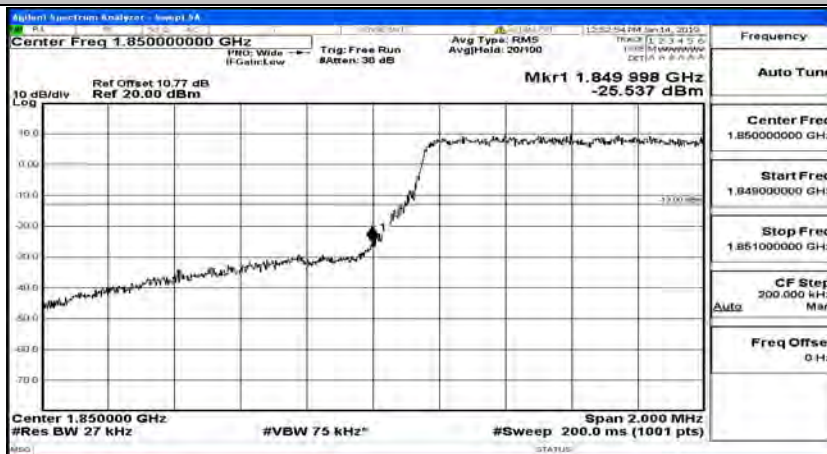
Band Edge Test Graph(s) (Channel Bandwidth: 1.4 MHz)_LCH_16QAM
