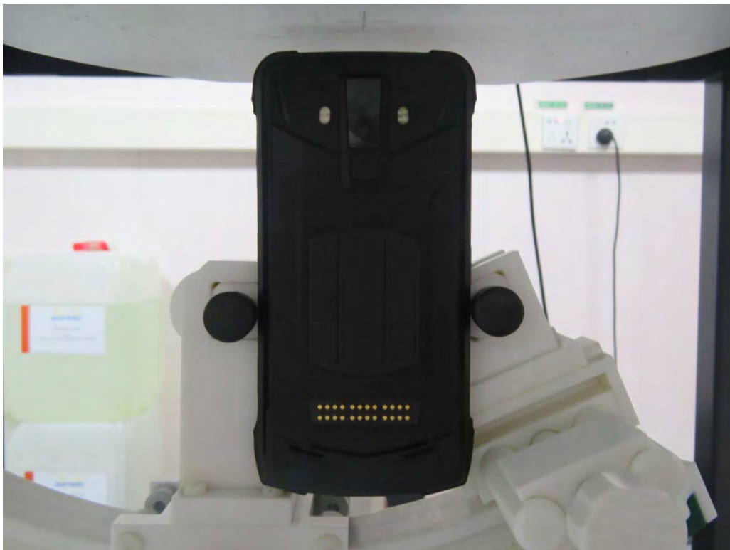
10mm body-worn Top Side Setup Photo (hotspot)
