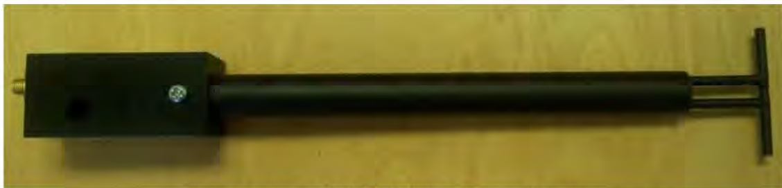
Figure 1 – MVG COMOSAR Validation Dipole
