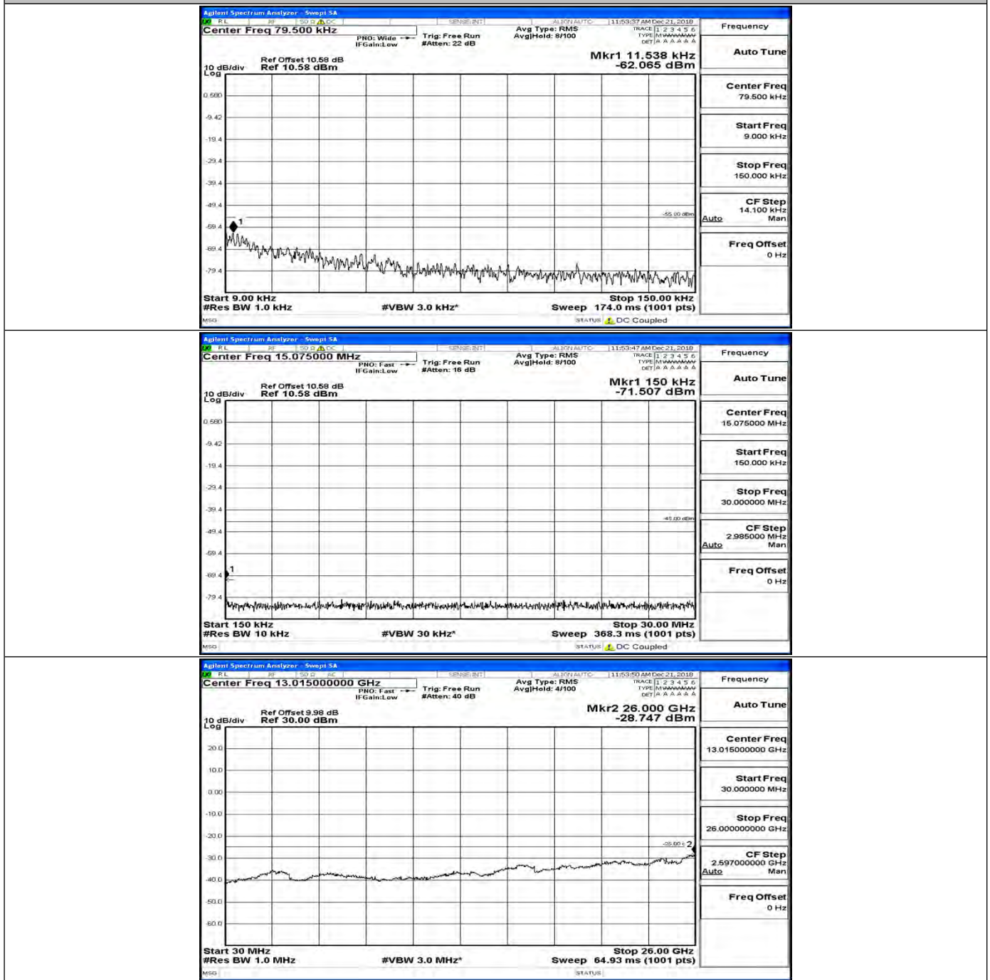
CSE Test Graph(s) (Channel Bandwidth: 5 MHz)_LCH_QPSK
