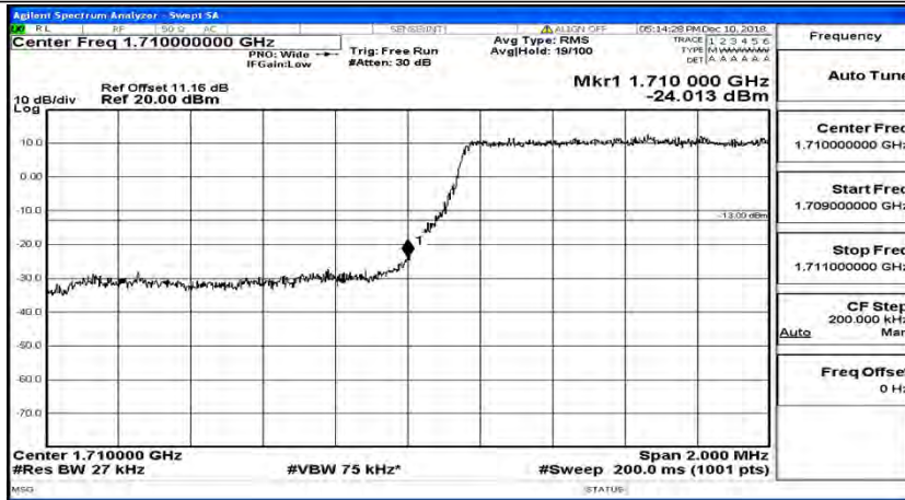
Band Edge Test Graph(s) (Channel Bandwidth: 1.4 MHz)_LCH_QPSK
