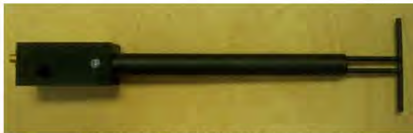
Figure 1 – MVG COMOSAR Validation Dipole
