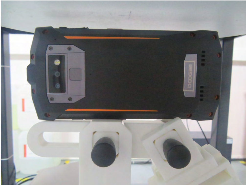
10mm body-worn Left Side Setup Photo (hotspot)
