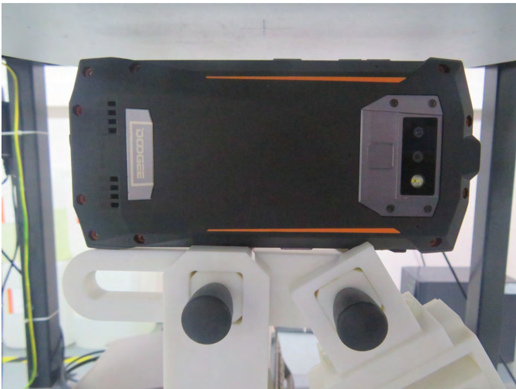
10mm body-worn Right Side Setup Photo (hotspot)
