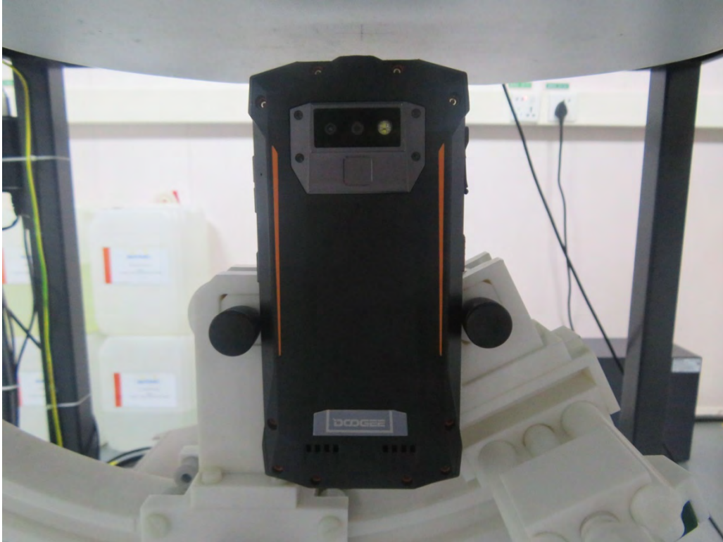
10mm body-worn Top Side Setup Photo (hotspot)
