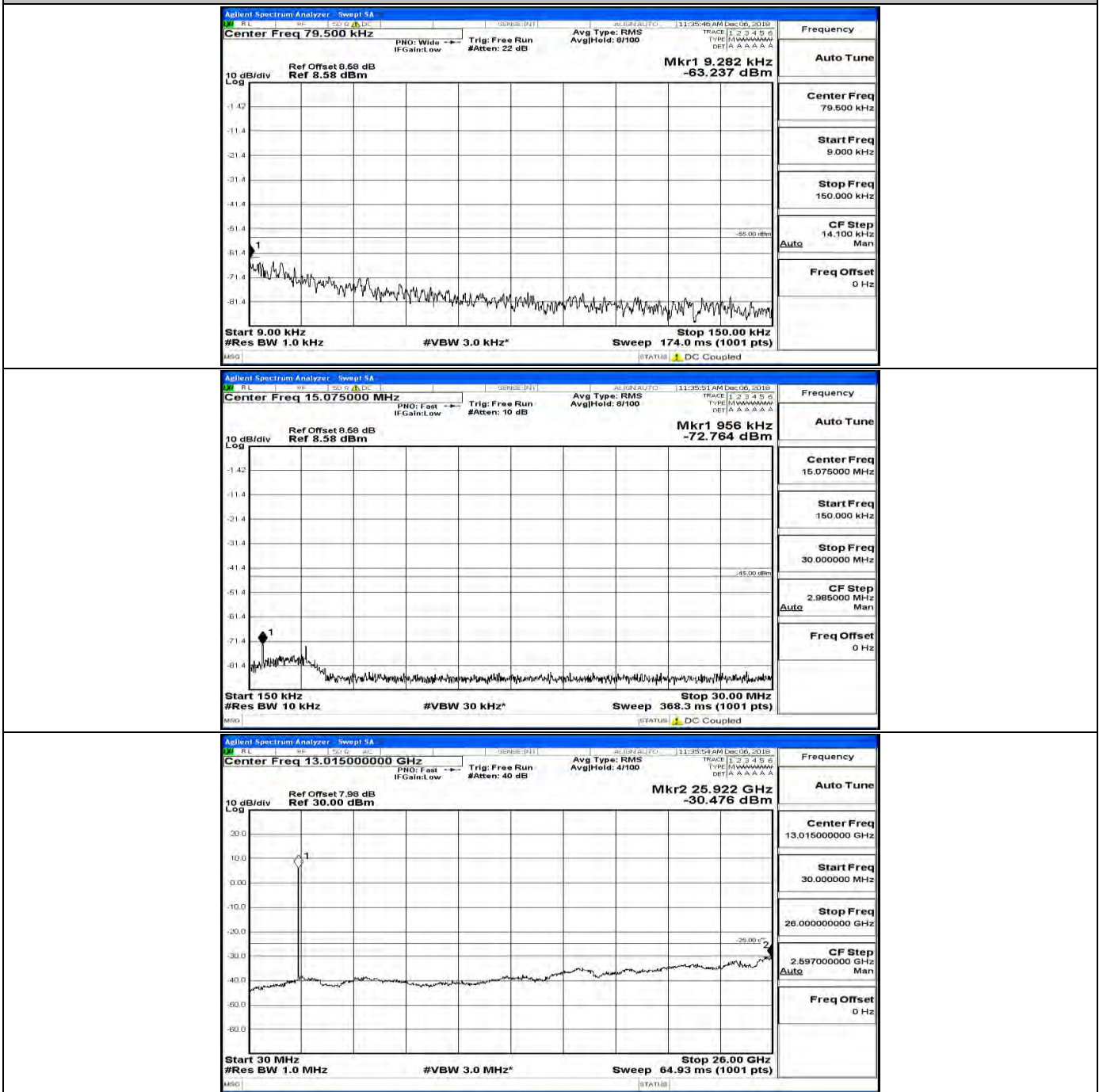
CSE Test Graph(s) (Channel Bandwidth: 5 MHz)_LCH_QPSK
