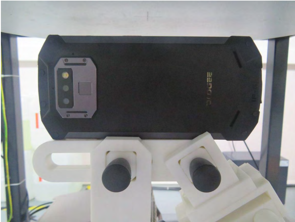
10mm body-worn Left Side Setup Photo (hotspot)
