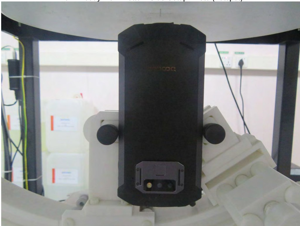
10mm body-worn Bottom Side Setup Photo (hotspot)
