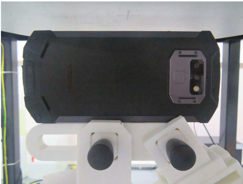
10mm body-worn Right Side Setup Photo (hotspot)
