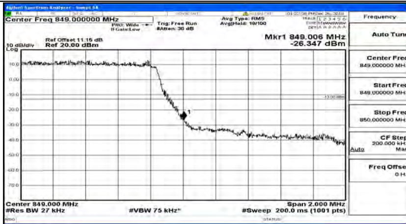
Band Edge Test Graph(s) (Channel Bandwidth: 1.4 MHz)_HCH_QPSK
