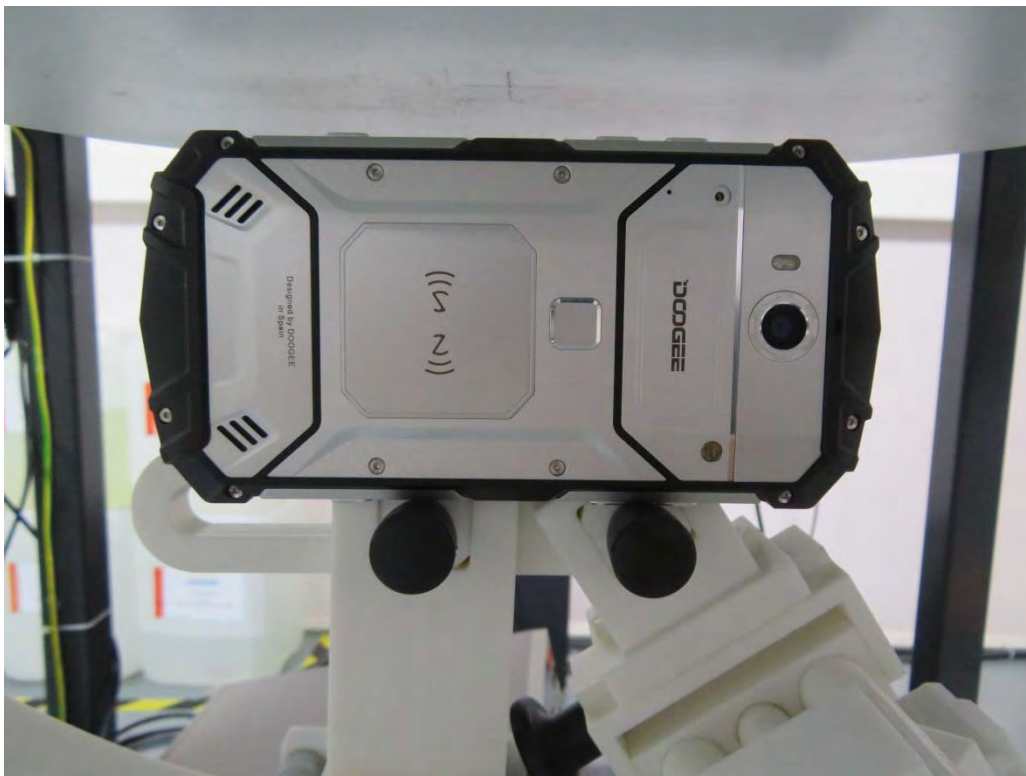
10mm body-worn Right Side Setup Photo (hotspot)
