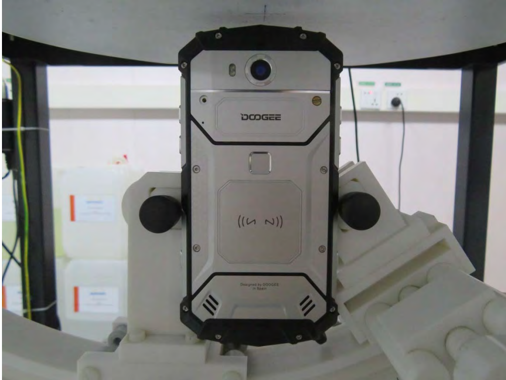
10mm body-worn Top Side Setup Photo (hotspot)
