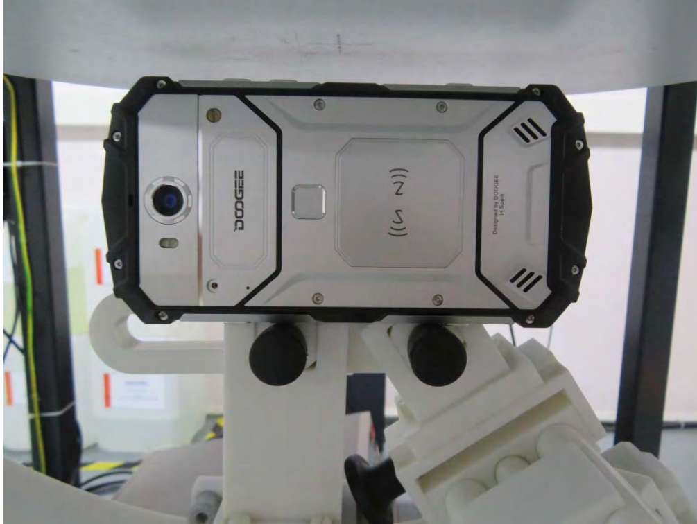
10mm body-worn Left Side Setup Photo (hotspot)
