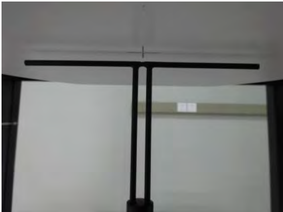
Photo of Dipole Setup
