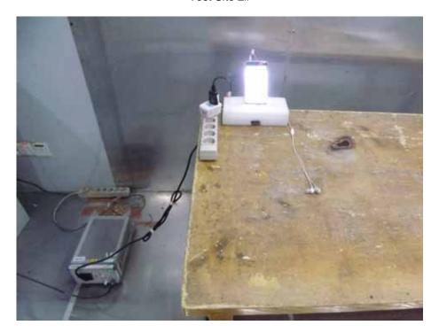
**Photograph - Spurious Emissions Radiated Test Setup**
