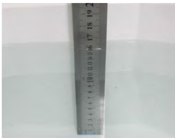
Liquid Height for Head SAR
