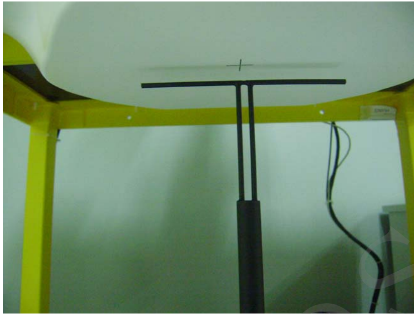
Setup Photo of Dipole Antenna
