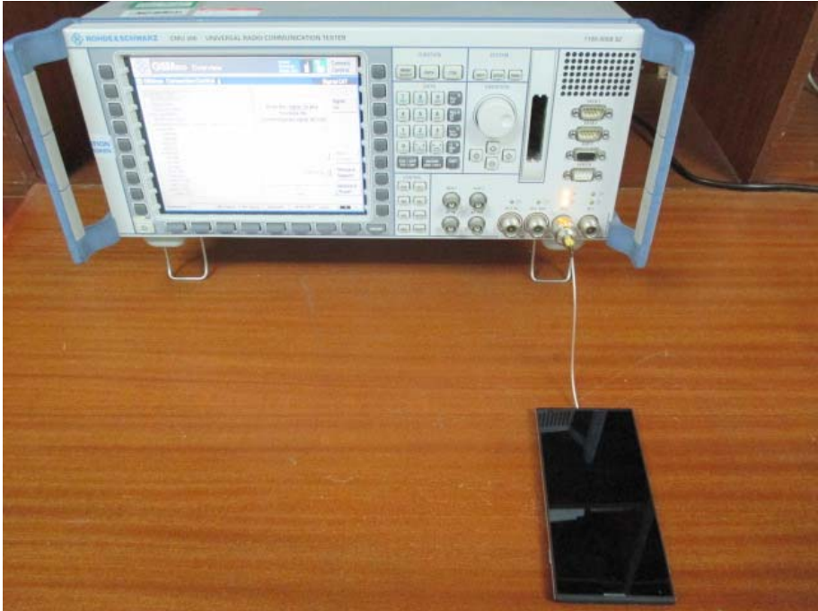
Photograph –2G&3G Conducted Test Setup
