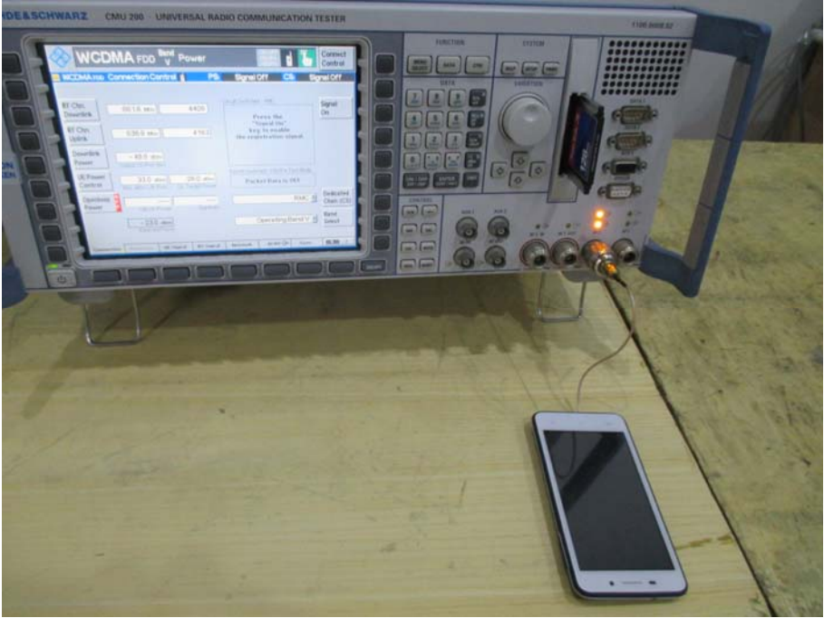
Photograph –2G&3G Conducted Test Setup
