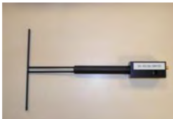
Figure 1 – Satimo COMOSAR Validation Dipole
