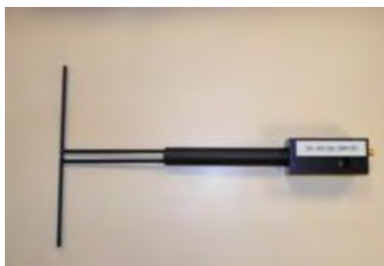
Figure 1 – Satimo COMOSAR Validation Dipole
