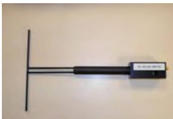
Figure 1 – Satimo COMOSAR Validation Dipole
