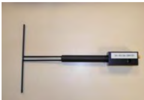
Figure 1 – Satimo COMOSAR Validation Dipole
