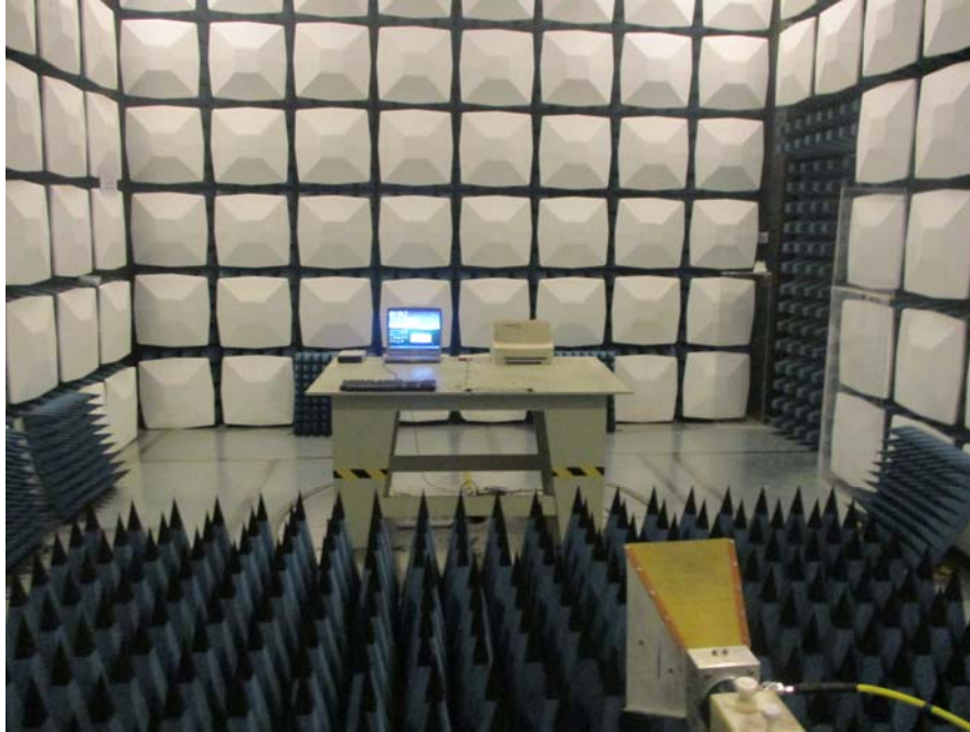
Radiated Emission Front View (Above 1GHz)
