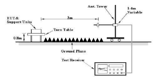
The radiated emission Below 1GHz tests were performed in the 3 meters chamber test site, above 1GHz tests were performed in the 3 meters chamber test site, using the setup accordance with the ANSI C63.4-2014. The specification used was the FCC Part 15.109 Class B limits.
