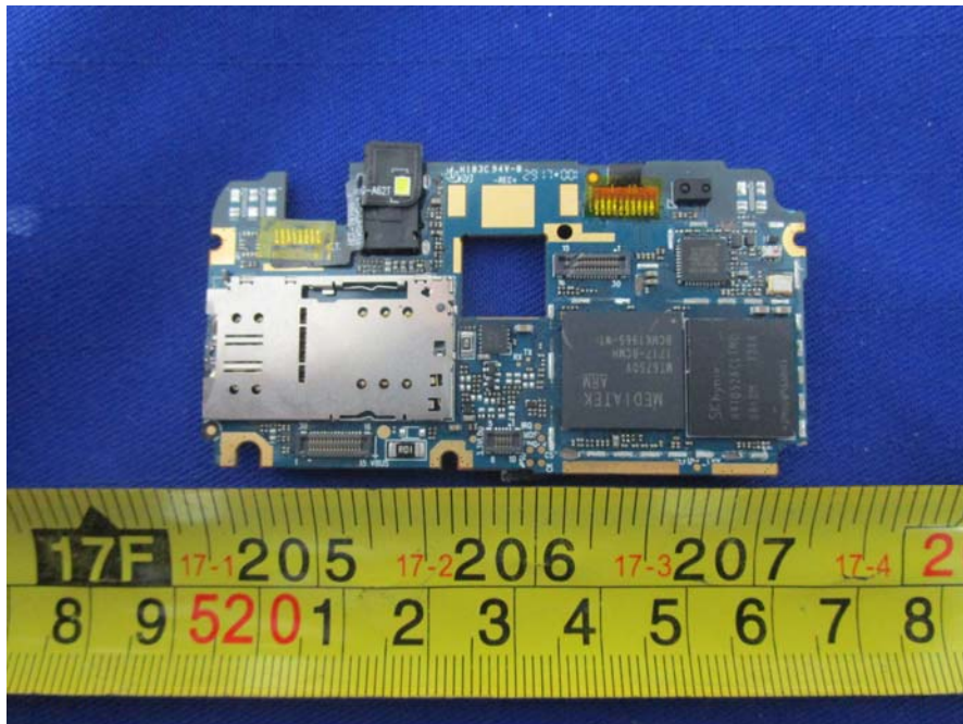
EUT – Main Board Unshield Top View
