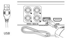
Output the USB mouse into the USB port on the back of the DVR.
