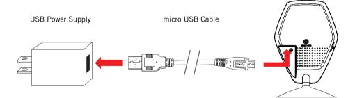
2 Plug the power supply into a socket or a UPS (Uninterruptible Power Supply).
