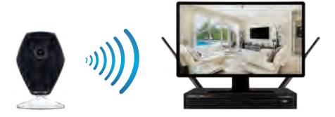
**NOTE:** If you see the camera(s) live view, you can move the camera(s) to the mounting location(s). If you no longer see the live view after moving the camera(s) to their mounting location, the camera may be too far from the DVR.
