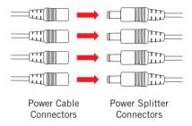
Connect the red female power leads of the video/power cables to the male power splitter ends.
