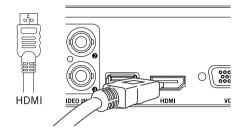
Plug included HDMI cable into the HDMI port on the back of the DVR.
