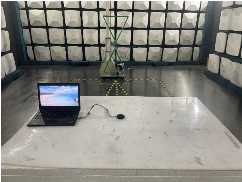
Radiated Spurious Emissions Test Setup 30MHz to 1GHz
