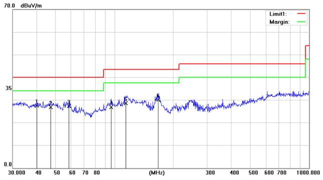
Test Mode: 00; Polarity: Horizontal; Modulation:GFSK; Channel:Low
