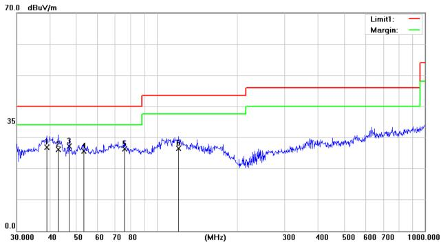
Test Mode: 00; Polarity: Vertical; Modulation:GFSK; Channel:Low
