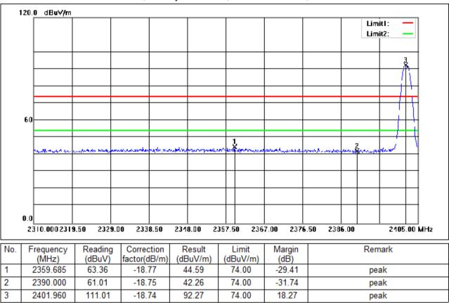
Test Mode: 00; Polarity: Horizontal; Modulation:GFSK; Channel:Low
