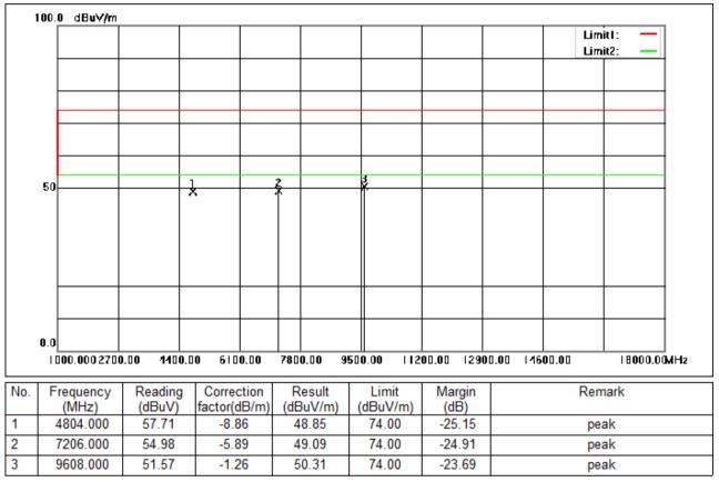
Test Mode: 00; Polarity: Vertical; Modulation:GFSK; Channel:Low
