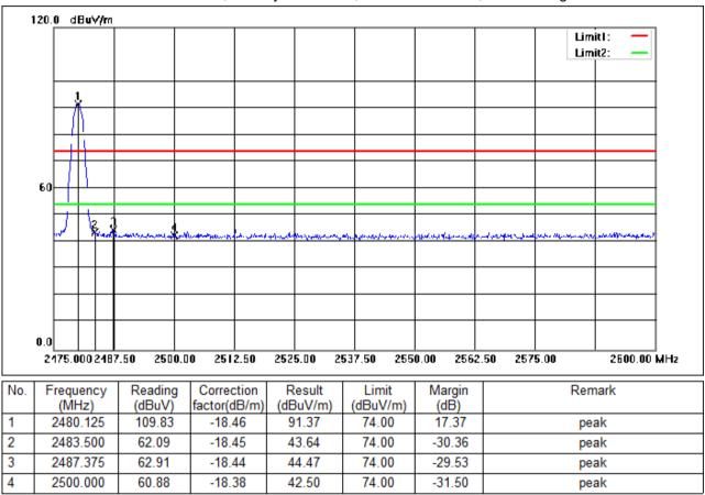
Test Mode: 00; Polarity: Horizontal; Modulation:GFSK; Channel:High
