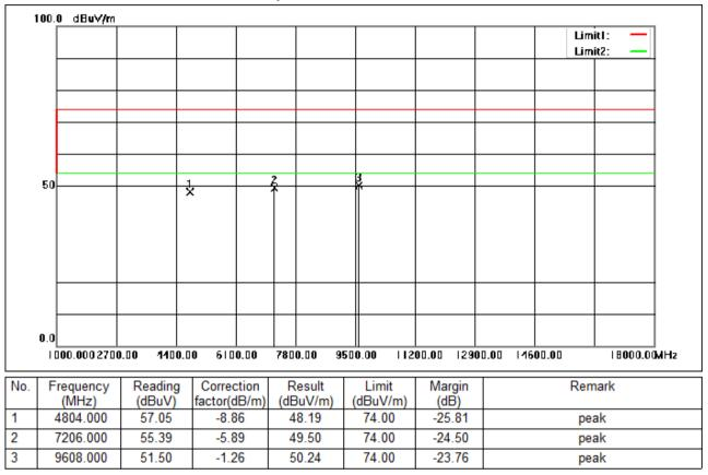
Test Mode: 00; Polarity: Horizontal; Modulation:GFSK; Channel:Low
