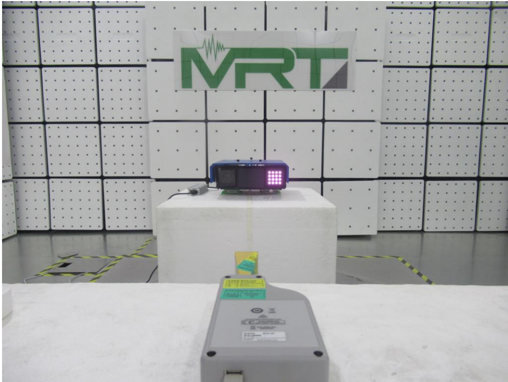
Description: Radiated Emission Test Setup for 75GHz ~ 100GHz
