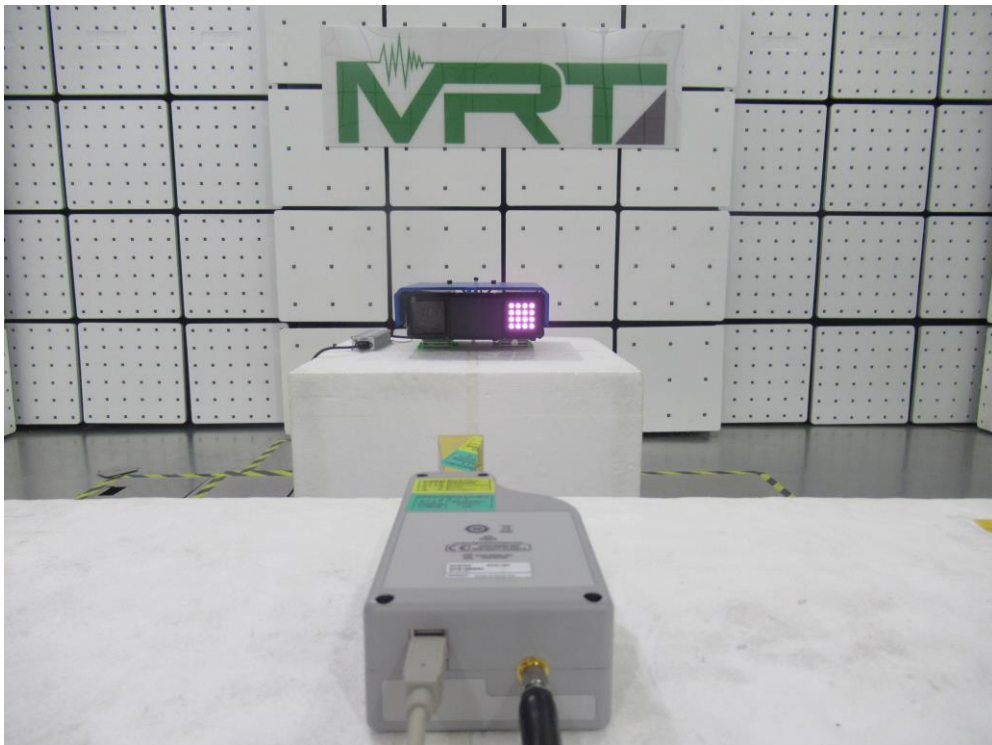
Description: Radiated Emission Test Setup for 75GHz ~ 100GHz
