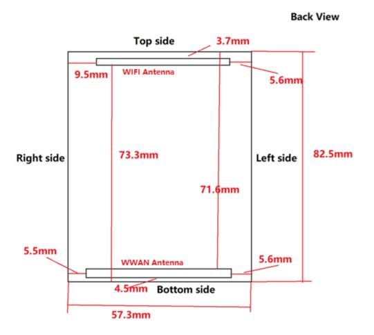
Distance from antenna to front side: 8.5mm Distance from antenna to Back side: 15mm
