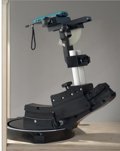
F-2. Device Holder for Transmitters
