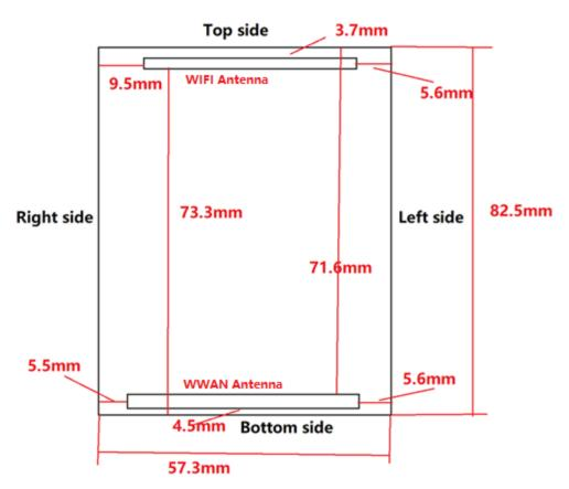
Distance from antenna to front side: 8.5mm Distance from antenna to Back side: 15mm
