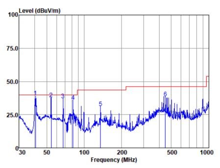
Antenna Polarity :VERTICAL Test mode :a
