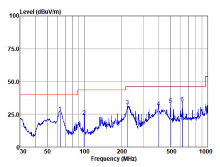
Antenna Polarity :VERTICAL EUT/Project :5210CR Test mode :a
