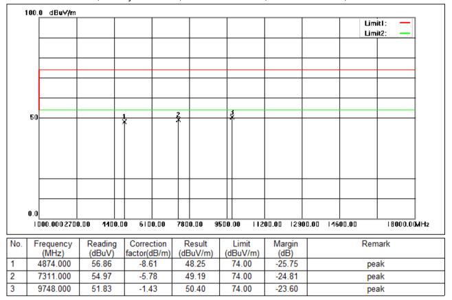
Test Mode: 00; Polarity: Horizontal; Modulation:802.11n; Bandwidth:40MHz; Channel:middle
