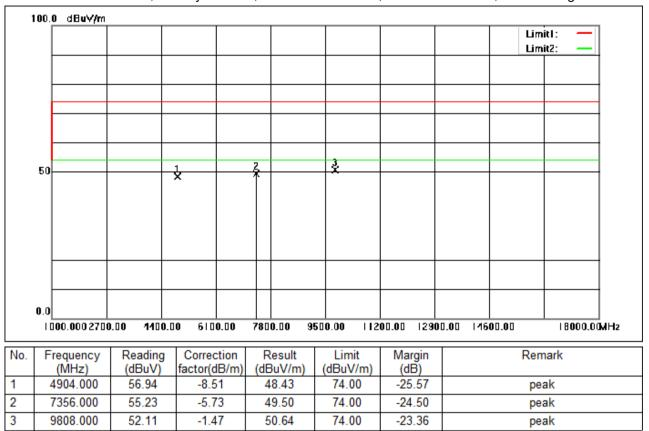
Test Mode: 00; Polarity: Vertical; Modulation:802.11n; Bandwidth:40MHz; Channel:High
