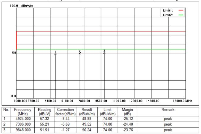
Test Mode: 00; Polarity: Vertical; Modulation:802.11n; Bandwidth:20MHz; Channel:High
