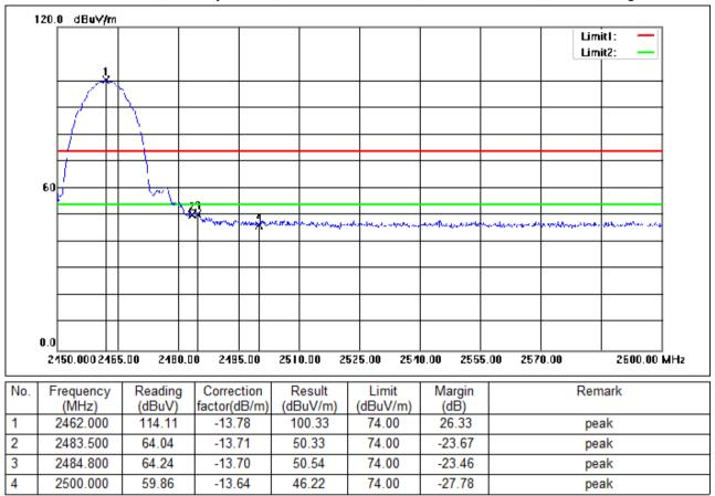
Test Mode: 00; Polarity: Vertical; Modulation:802.11b; Bandwidth:20MHz; Channel:High
