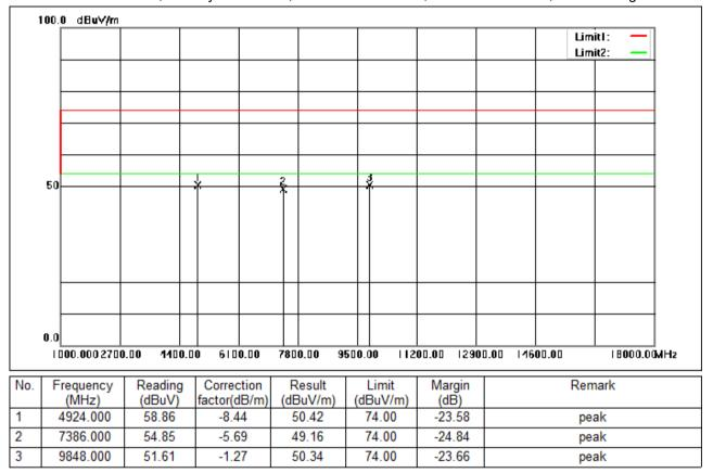
Test Mode: 00; Polarity: Horizontal; Modulation:802.11b; Bandwidth:20MHz; Channel:High
