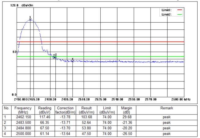
Test Mode: 00; Polarity: Horizontal; Modulation:802.11b; Bandwidth:20MHz; Channel:High
