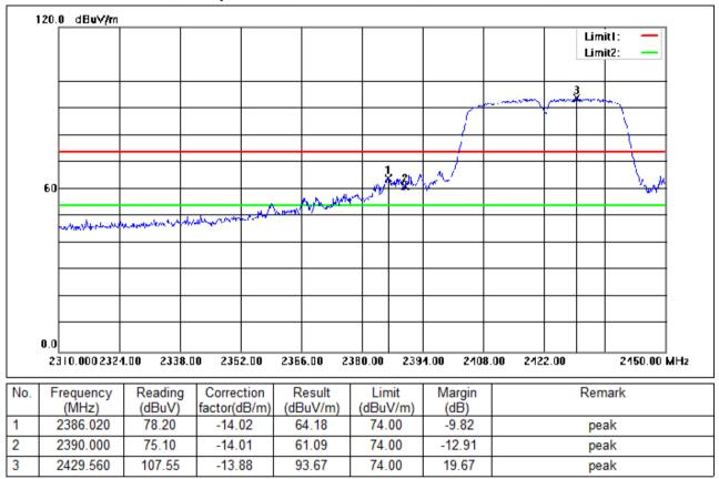
Test Mode: 00; Polarity: Vertical; Modulation:802.11n; Bandwidth:40MHz; Channel:Low
