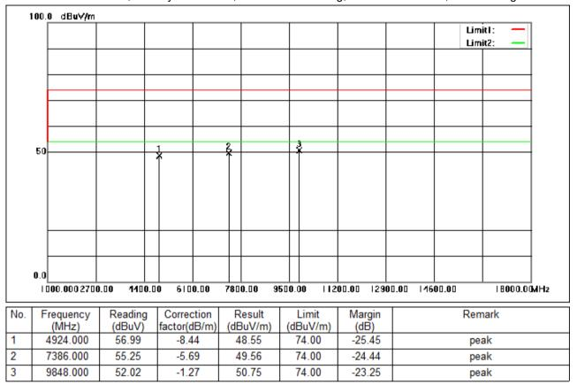
Test Mode: 00; Polarity: Horizontal; Modulation:802.11g; Bandwidth:20MHz; Channel:High
