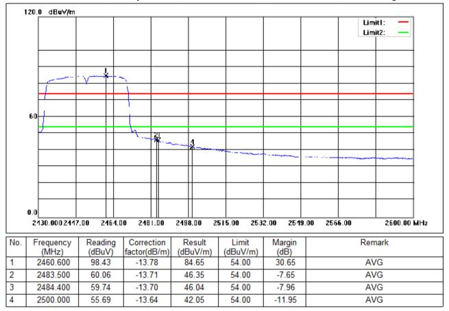
Test Mode: 00; Polarity: Vertical; Modulation:802.11n; Bandwidth:40MHz; Channel:High
