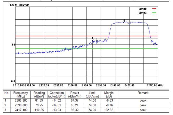
Test Mode: 00; Polarity: Horizontal; Modulation:802.11n; Bandwidth:40MHz; Channel:Low
