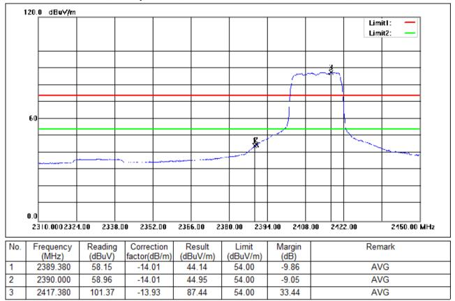
Test Mode: 00; Polarity: Vertical; Modulation:802.11n; Bandwidth:20MHz; Channel:Low
