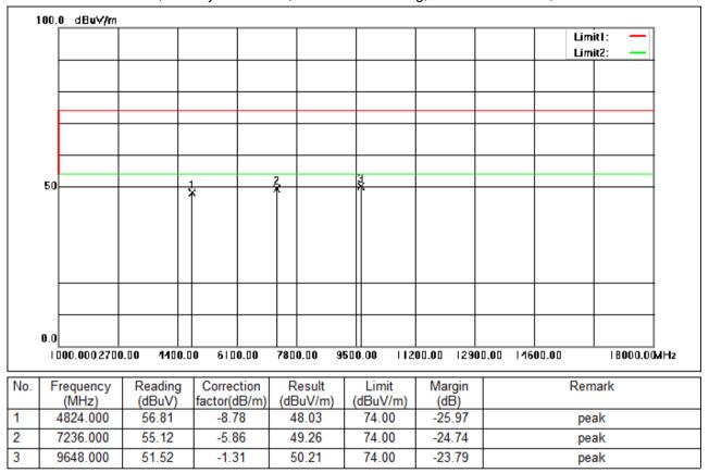
Test Mode: 00; Polarity: Horizontal; Modulation:802.11g; Bandwidth:20MHz; Channel:Low
