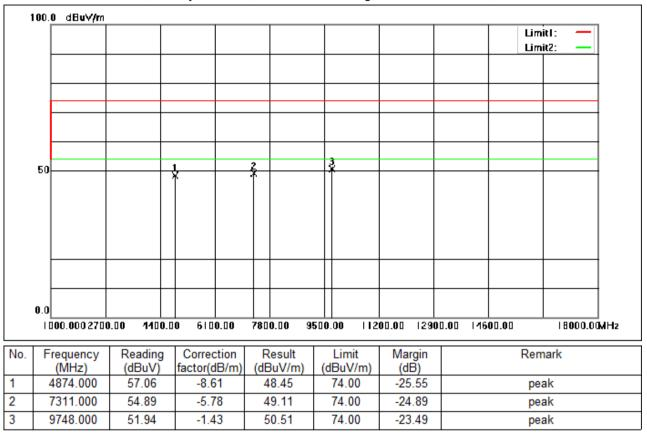
Test Mode: 00; Polarity: Vertical; Modulation:802.11g; Bandwidth:20MHz; Channel:middle
