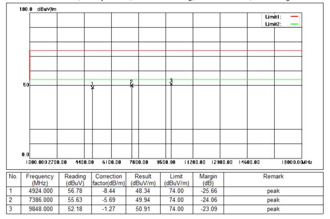
Test Mode: 00; Polarity: Vertical; Modulation:802.11g; Bandwidth:20MHz; Channel:High
