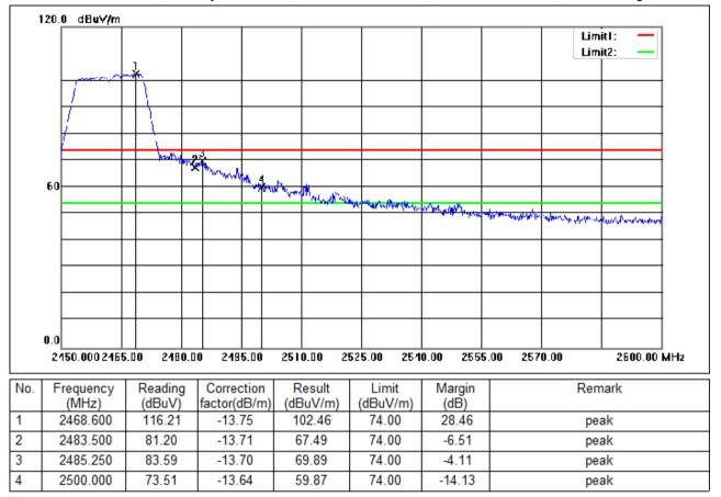
Test Mode: 00; Polarity: Horizontal; Modulation:802.11n; Bandwidth:20MHz; Channel:High
