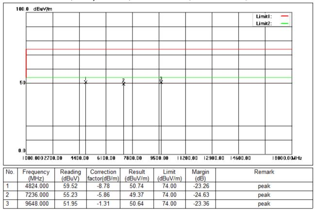
Test Mode: 00; Polarity: Horizontal; Modulation:802.11b; Bandwidth:20MHz; Channel:Low
