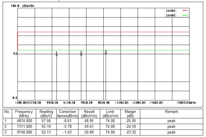
Test Mode: 00; Polarity: Horizontal; Modulation:802.11n; Bandwidth:20MHz; Channel:middle
