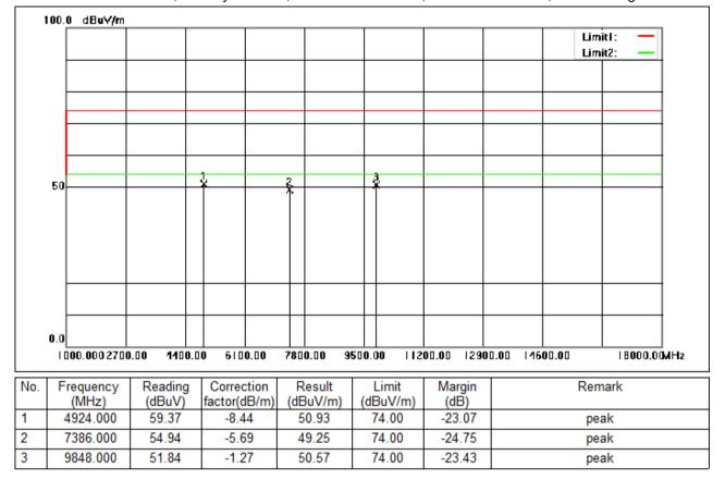
Test Mode: 00; Polarity: Vertical; Modulation:802.11b; Bandwidth:20MHz; Channel:High
