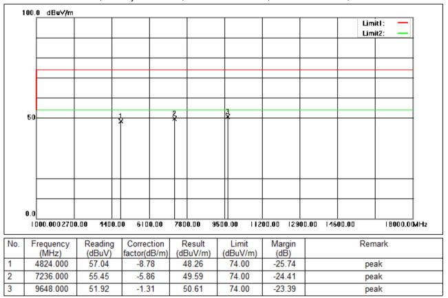
Test Mode: 00; Polarity: Horizontal; Modulation:802.11n; Bandwidth:20MHz; Channel:Low
