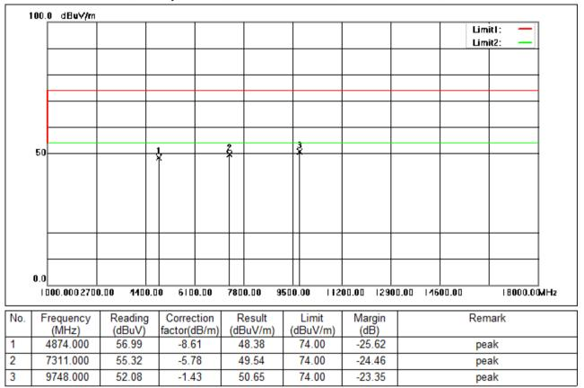
Test Mode: 00; Polarity: Vertical; Modulation:802.11n; Bandwidth:20MHz; Channel:middle
