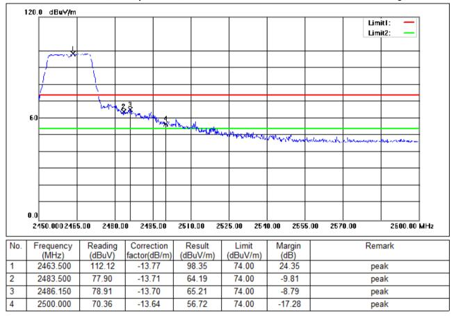
Test Mode: 00; Polarity: Vertical; Modulation:802.11n; Bandwidth:20MHz; Channel:High
