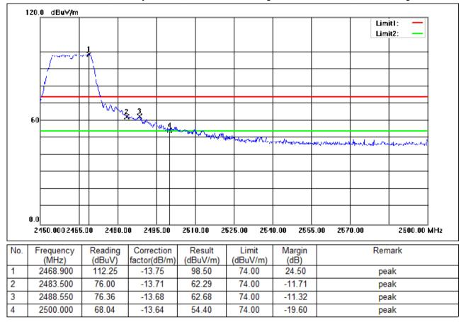
Test Mode: 00; Polarity: Vertical; Modulation:802.11g; Bandwidth:20MHz; Channel:High
