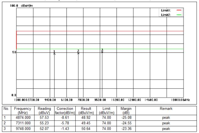
Test Mode: 00; Polarity: Vertical; Modulation:802.11n; Bandwidth:40MHz; Channel:middle
