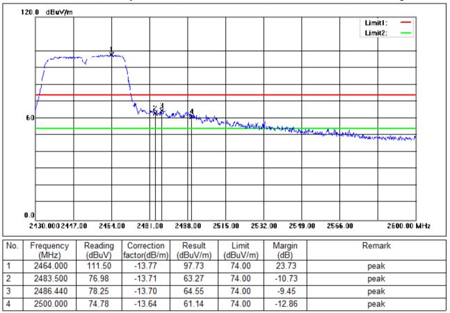
Test Mode: 00; Polarity: Horizontal; Modulation:802.11n; Bandwidth:40MHz; Channel:High
