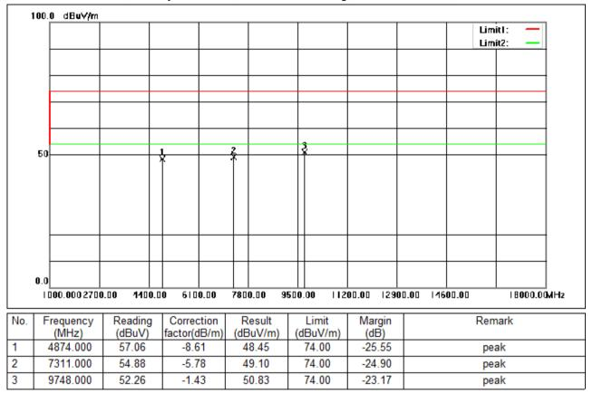
Test Mode: 00; Polarity: Horizontal; Modulation:802.11g; Bandwidth:20MHz; Channel:middle
