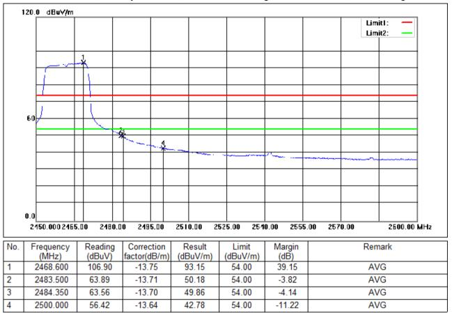
Test Mode: 00; Polarity: Horizontal; Modulation:802.11g; Bandwidth:20MHz; Channel:High
