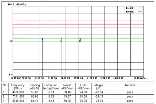
Test Mode: 00; Polarity: Vertical; Modulation:802.11b; Bandwidth:20MHz; Channel:middle
