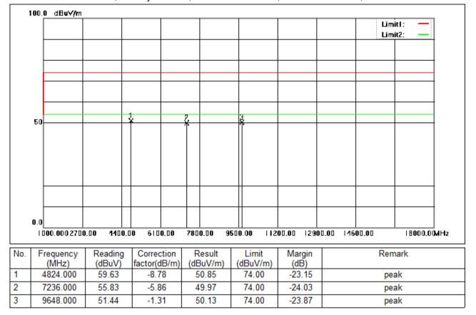
Test Mode: 00; Polarity: Vertical; Modulation:802.11b; Bandwidth:20MHz; Channel:Low
