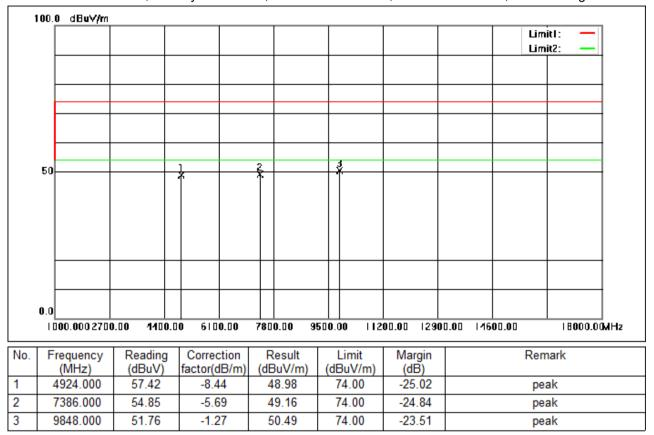
Test Mode: 00; Polarity: Horizontal; Modulation:802.11n; Bandwidth:20MHz; Channel:High
