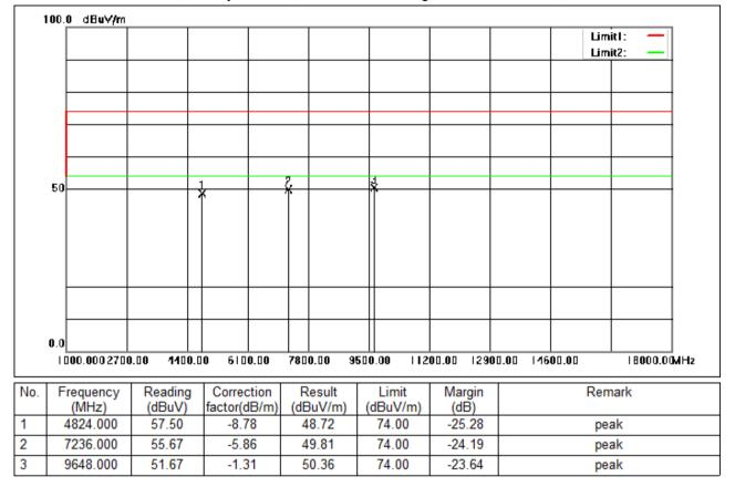
Test Mode: 00; Polarity: Vertical; Modulation:802.11g; Bandwidth:20MHz; Channel:Low
