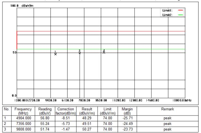
Test Mode: 00; Polarity: Horizontal; Modulation:802.11n; Bandwidth:40MHz; Channel:High
