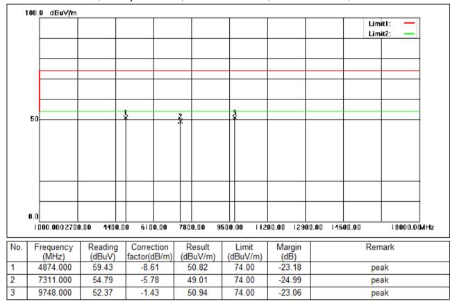
Test Mode: 00; Polarity: Horizontal; Modulation:802.11b; Bandwidth:20MHz; Channel:middle
