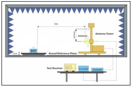
Limit: The bandwidth of the emission shall be no wider than 0.25% of the center frequency for devices operating above 70 MHz and below 900 MHz. For devices operating above 900 MHz, the emission shall be no wider than 0.5% of the center frequency. Bandwidth is determined at the points 20 dB down from the modulated carrier.
