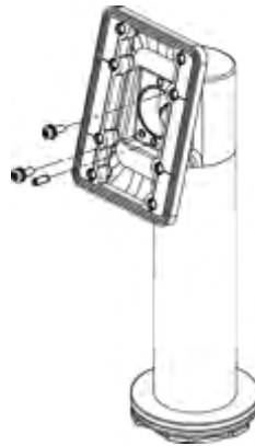
Figure 3-11 Take off Screws
