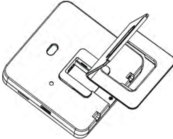
Figure 3-4 Place Bracket Close to Device Back Side
