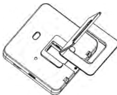
Figure 3-4 Place Bracket Close to Device Back Side
