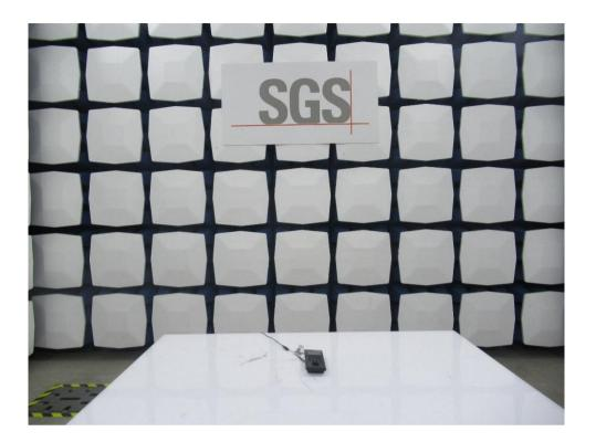
Radiated Emissions (9kHz-30MHz)
