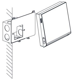
Figure 3-7 Buckle Terminal on Plate
