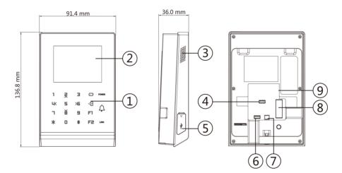
Figure 2-1 Diagram of Access Control Terminal Appearance (Without Fingerprint Module) Table 2-1 Description of Access Control Terminal (Without Fingerprint Module)
