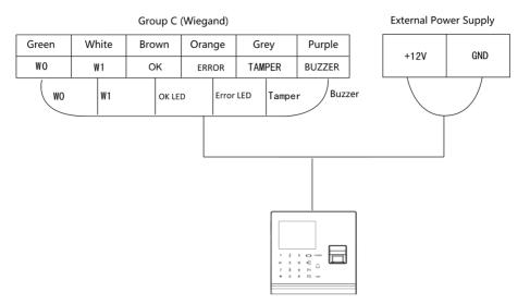
Figure 4-6 Wiring as Wiegand Card Reader
