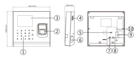
Figure 2-2 Diagram of Access Control Terminal Appearance (With Fingerprint Module)
