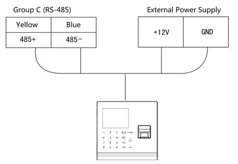
Figure 4-5 Wiring of RS-485 Output
