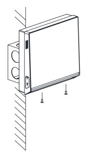
Figure 3-8 Tighten Screws
