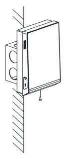
Figure 3-4 Tighten Screw
