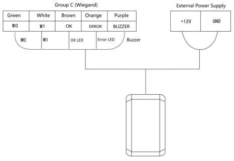
Figure 4-4 Wiring of Wiegand Card Reader
