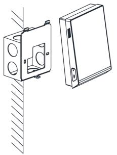
Figure 3-3 Buckle Terminal on Plate
