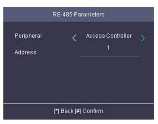
Figure 6-6 Set RS-485 Parameters
