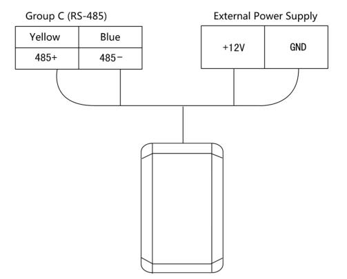
Figure 4-3 Wiring of External RS-485 Card Reader
