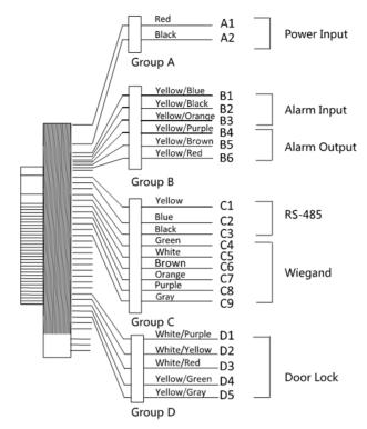
Figure 4-1 Terminal Diagram
