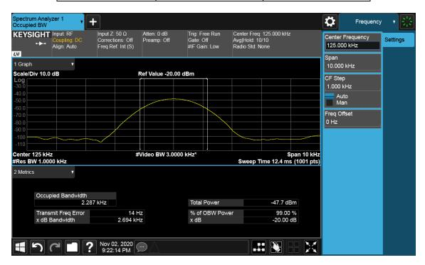
Remark: Because the measured signal is CW or CW-like adjusting the RBW per C63.10 would not be practical since measured bandwidth will always follow the RBW and the result will be approximately twice the RBW. And the signal was narrowband, therefore it was impossible to set RBW within 1% - 5%.
