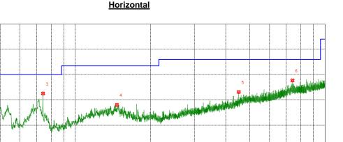
Reading No. Frequency **Factor** Result Limit Margin Remark (MHz) [dBµV/m] [dB] (dBuV/m) (dBuV/m) (dB) -5.97 20.37 40.6711 13.66 34.03 40.00 peak 2 40.00 47.7528 16.61 16.05 32.66 -7.34 peak 3 74.2364 17.82 14.77 32.59 40.00 -7.41 peak 146,7997 19.82 43.50 -15.38 4 8.30 28.12 peak 5 -12.84 451.6042 8.54 24.62 33.16 46.00 peak 6 741.1781 8.71 29.02 37.73 46.00 -8.27 peak
