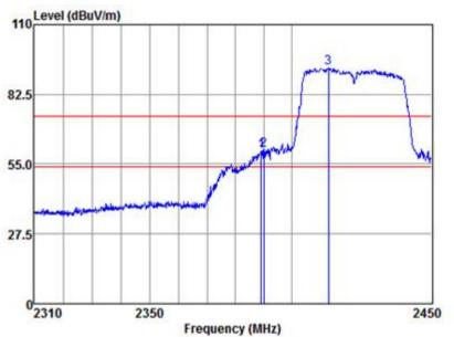
Mode:a; Polarization:Horizontal; Modulation:n; bandwidth:40MHz; Channel:Low
