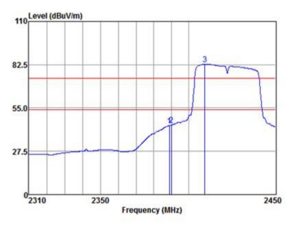
Mode:a; Polarization:Horizontal; Modulation:n; bandwidth:40MHz; Channel:Low
