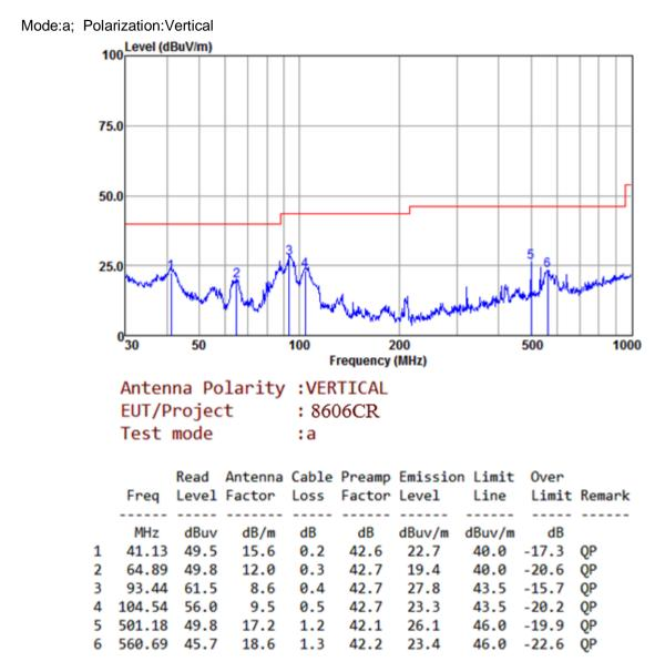
Note:Emission Level=Read Level+Antenna Factor+Cable loss-Preamp Factor
