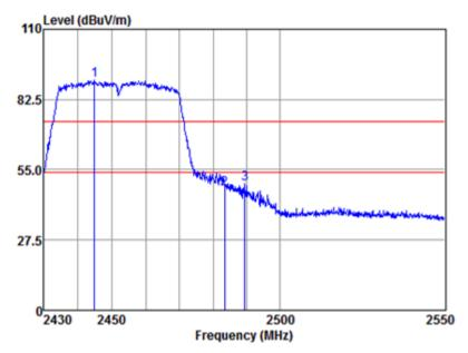
Mode:a; Polarization:Vertical; Modulation:n; bandwidth:40MHz; Channel:High
