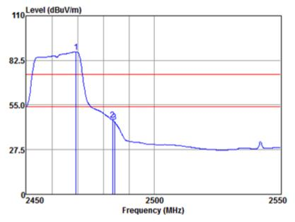
Mode:a; Polarization:Horizontal; Modulation:n; bandwidth:20MHz; Channel:High
