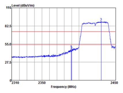
Mode:a; Polarization:Vertical; Modulation:n; bandwidth:40MHz; Channel:Low
