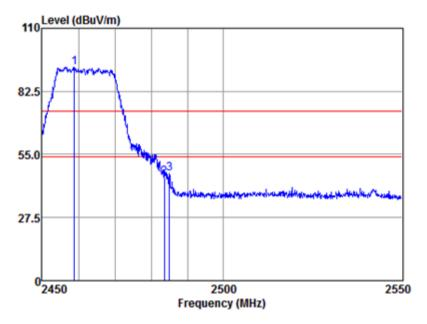
Mode:a; Polarization:Vertical; Modulation:g; bandwidth:20MHz; Channel:High
