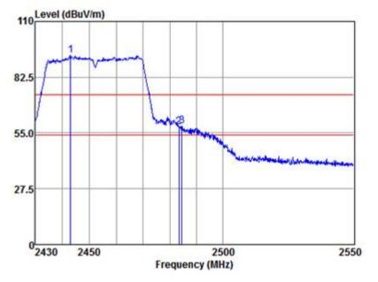
Mode:a; Polarization:Horizontal; Modulation:n; bandwidth:40MHz; Channel:High
