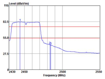
Mode:a; Polarization:Horizontal; Modulation:n; bandwidth:40MHz; Channel:High
