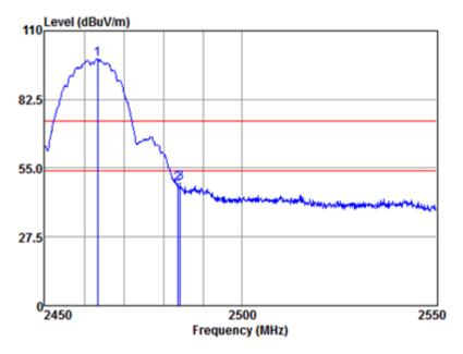
Mode:a; Polarization:Horizontal; Modulation:b; bandwidth:20MHz; Channel:High
