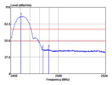
Mode:a; Polarization:Vertical; Modulation:b; bandwidth:20MHz; Channel:High
