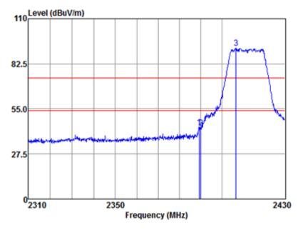
Mode:a; Polarization:Vertical; Modulation:g; bandwidth:20MHz; Channel:Low
