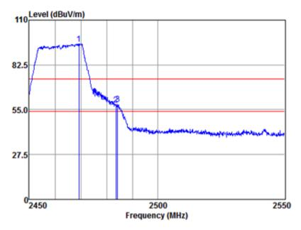
Mode:a; Polarization:Horizontal; Modulation:n; bandwidth:20MHz; Channel:High
