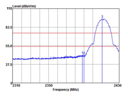
Mode:a; Polarization:Vertical; Modulation:b; bandwidth:20MHz; Channel:Low
