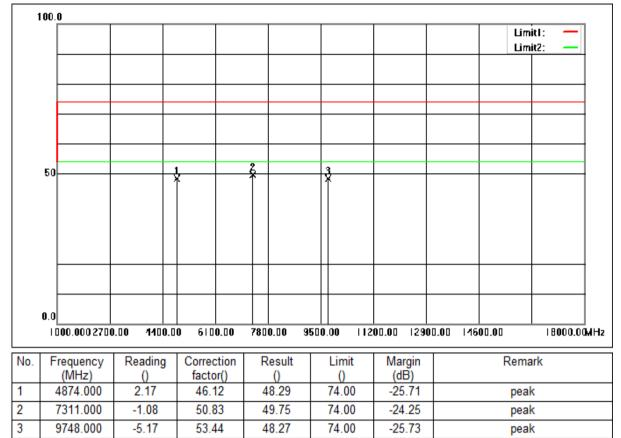
Mode:a; Polarization:Horizontal; Modulation:b; bandwidth:20MHz; Channel:middle
