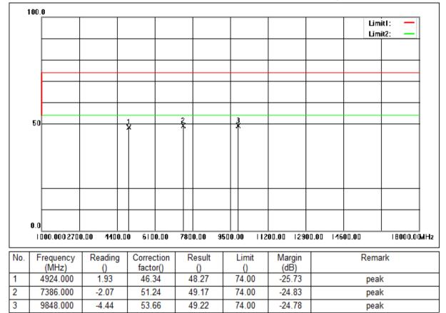
Mode:a; Polarization:Vertical; Modulation:b; bandwidth:20MHz; Channel:High
