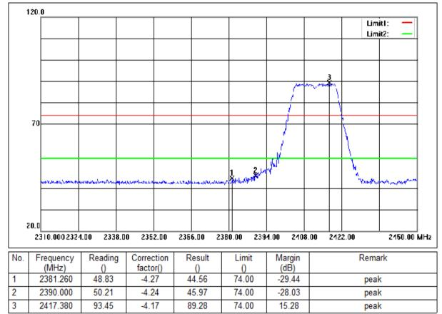
Mode:a; Polarization:Vertical; Modulation:n; bandwidth:20MHz; Channel:Low
