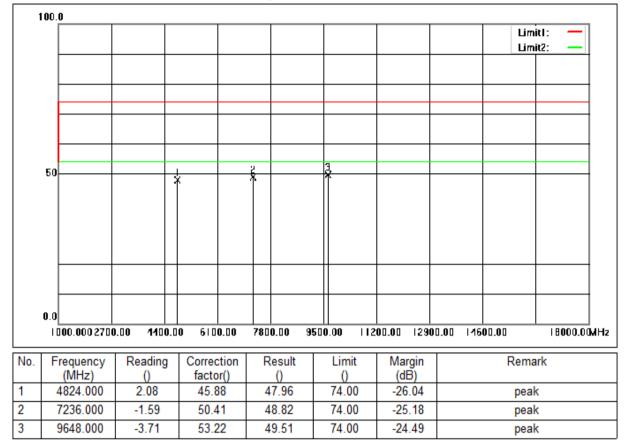
Mode:a; Polarization:Vertical; Modulation:g; bandwidth:20MHz; Channel:Low
