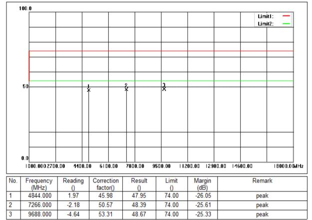
Mode:a; Polarization:Horizontal; Modulation:n; bandwidth:40MHz; Channel:Low
