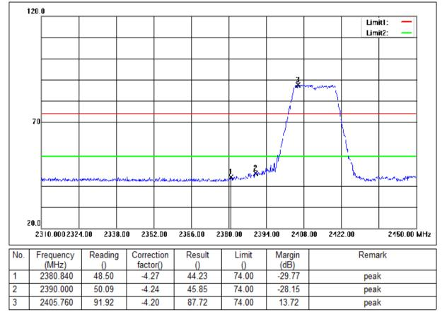
Mode:a; Polarization:Horizontal; Modulation:n; bandwidth:20MHz; Channel:Low
