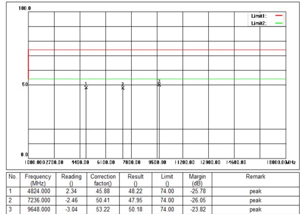
Mode:a; Polarization:Vertical; Modulation:b; bandwidth:20MHz; Channel:Low
