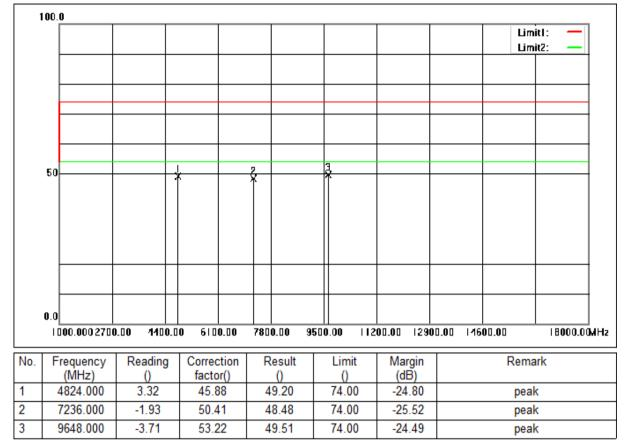
Mode:a; Polarization:Vertical; Modulation:n; bandwidth:20MHz; Channel:Low
