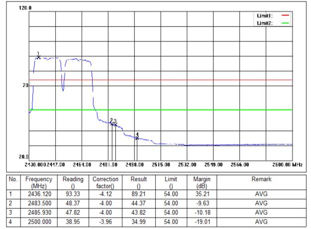
Mode:a; Polarization:Horizontal; Modulation:n; bandwidth:40MHz; Channel:High
