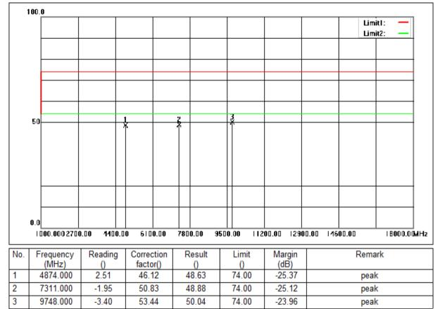
Mode:a; Polarization:Vertical; Modulation:n; bandwidth:20MHz; Channel:middle
