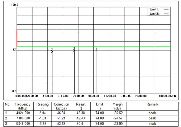
Mode:a; Polarization:Horizontal; Modulation:n; bandwidth:20MHz; Channel:High
