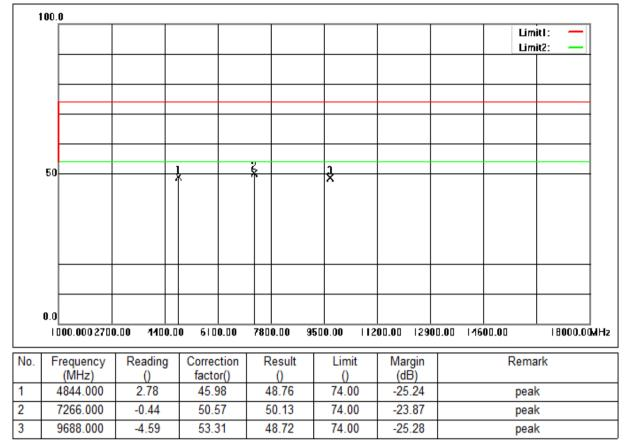
Mode:a; Polarization:Vertical; Modulation:n; bandwidth:40MHz; Channel:Low
