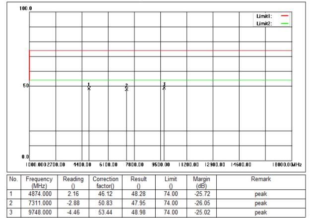
Mode:a; Polarization:Horizontal; Modulation:g; bandwidth:20MHz; Channel:middle
