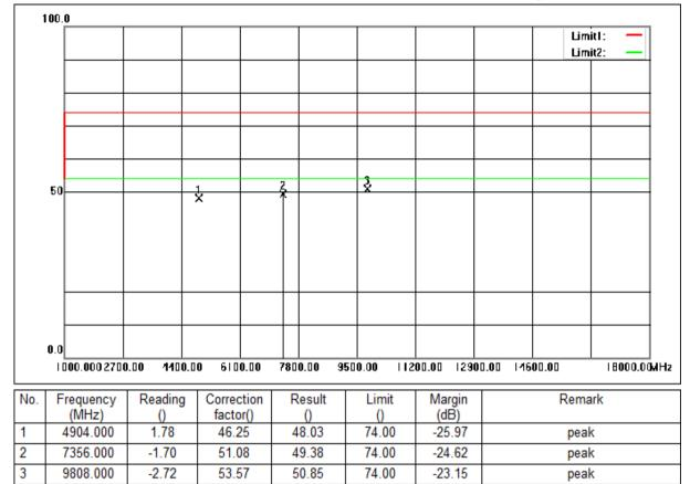
Mode:a; Polarization:Horizontal; Modulation:n; bandwidth:40MHz; Channel:High
