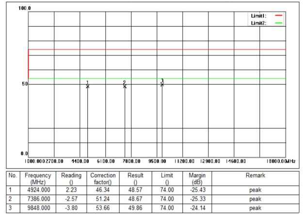
Mode:a; Polarization:Vertical; Modulation:g; bandwidth:20MHz; Channel:High
