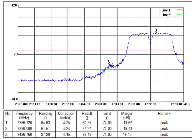
Mode:a; Polarization:Vertical; Modulation:n; bandwidth:40MHz; Channel:Low
