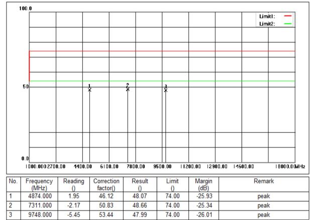
Mode:a; Polarization:Vertical; Modulation:n; bandwidth:40MHz; Channel:middle
