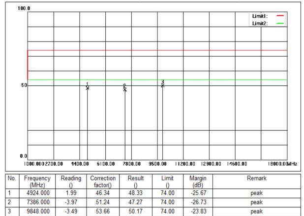
Mode:a; Polarization:Horizontal; Modulation:g; bandwidth:20MHz; Channel:High
