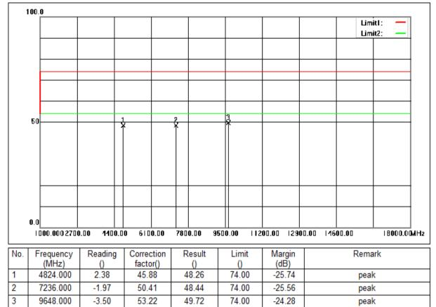
Mode:a; Polarization:Horizontal; Modulation:n; bandwidth:20MHz; Channel:Low
