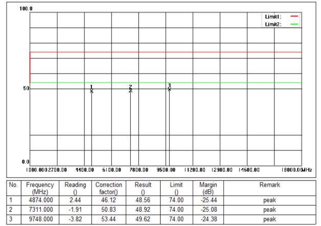
Mode:a; Polarization:Horizontal; Modulation:n; bandwidth:20MHz; Channel:middle
