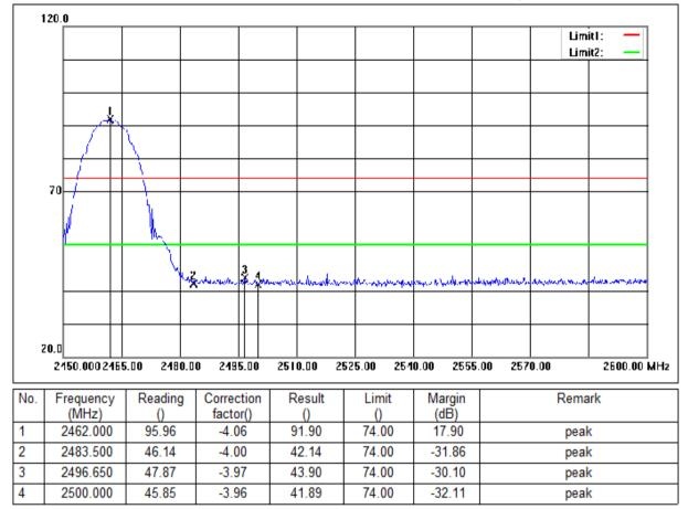
Mode:a; Polarization:Vertical; Modulation:b; bandwidth:20MHz; Channel:High
