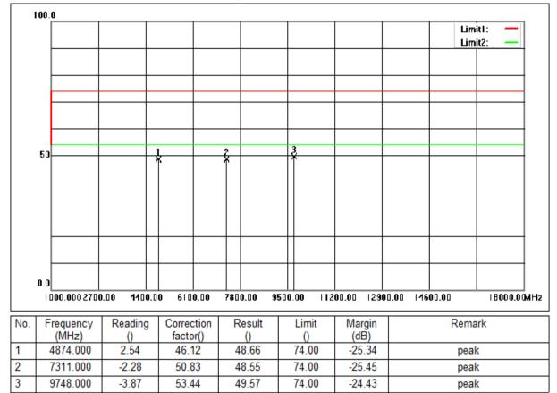
Mode:a; Polarization:Vertical; Modulation:g; bandwidth:20MHz; Channel:middle
