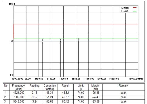
Mode:a; Polarization:Horizontal; Modulation:b; bandwidth:20MHz; Channel:High
