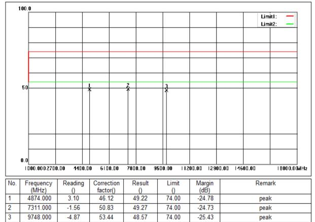
Mode:a; Polarization:Vertical; Modulation:b; bandwidth:20MHz; Channel:middle
