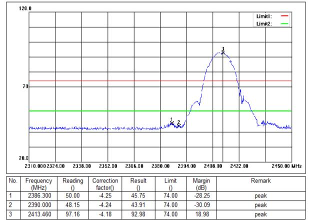
Mode:a; Polarization:Horizontal; Modulation:b; bandwidth:20MHz; Channel:Low
