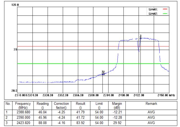
Mode:a; Polarization:Vertical; Modulation:n; bandwidth:40MHz; Channel:Low
