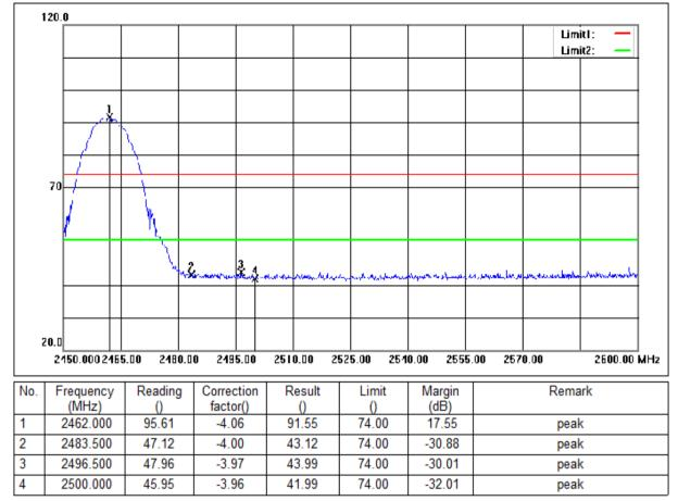
Mode:a; Polarization:Horizontal; Modulation:b; bandwidth:20MHz; Channel:High
