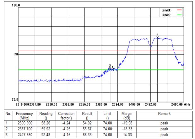
Mode:a; Polarization:Horizontal; Modulation:n; bandwidth:40MHz; Channel:Low
