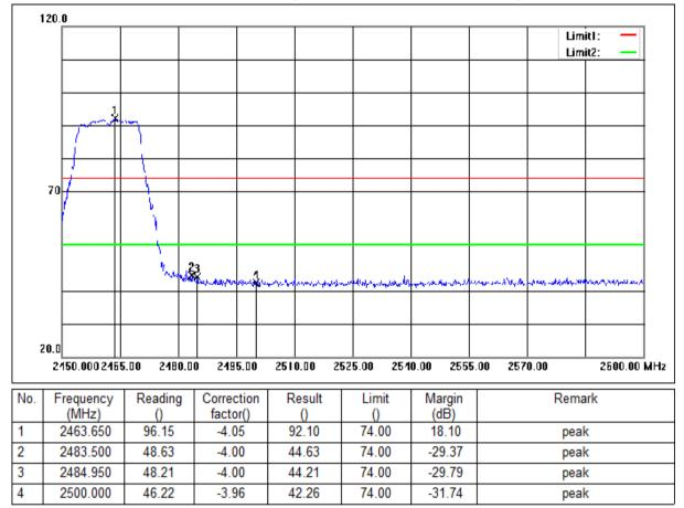
Mode:a; Polarization:Vertical; Modulation:g; bandwidth:20MHz; Channel:High
