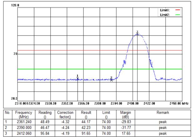
Mode:a; Polarization:Vertical; Modulation:b; bandwidth:20MHz; Channel:Low
