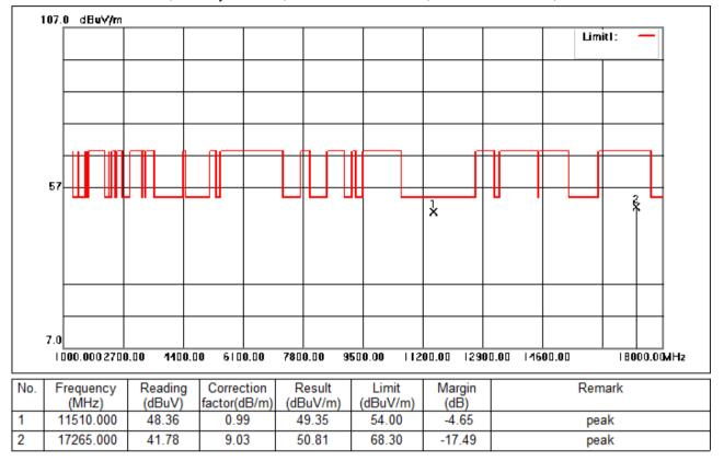
Test Mode: 06; Polarity: Vertical; Modulation:802.11ac; Bandwidth:40MHz; Channel:Low
