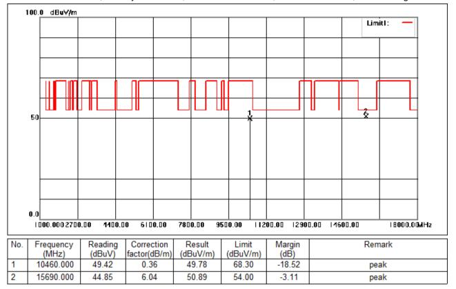
Test Mode: 05; Polarity: Horizontal; Modulation:802.11ac; Bandwidth:40MHz; Channel:High
