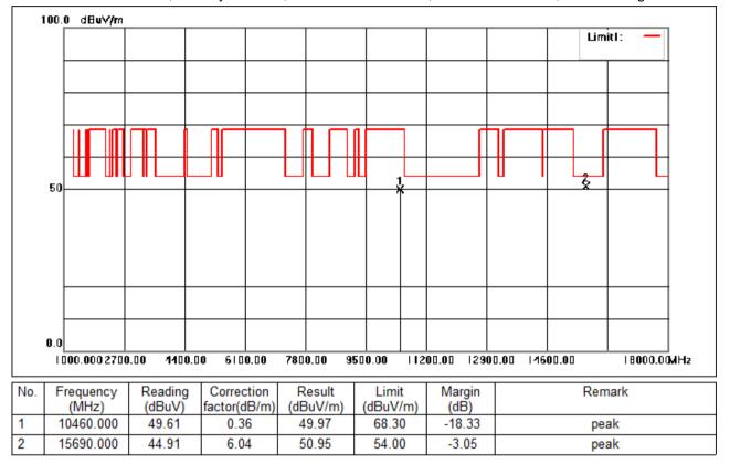
Test Mode: 05; Polarity: Vertical; Modulation:802.11ac; Bandwidth:40MHz; Channel:High
