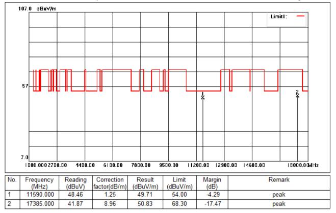
Test Mode: 06; Polarity: Horizontal; Modulation:802.11ac; Bandwidth:40MHz; Channel:High
