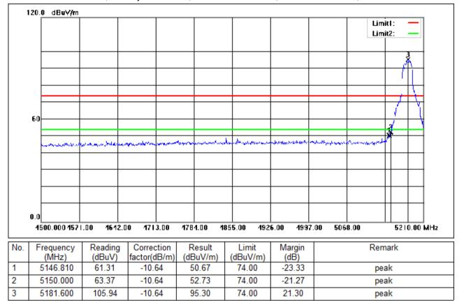
Test Mode: 05; Polarity: Horizontal; Modulation:802.11n; Bandwidth:20MHz; Channel:Low
