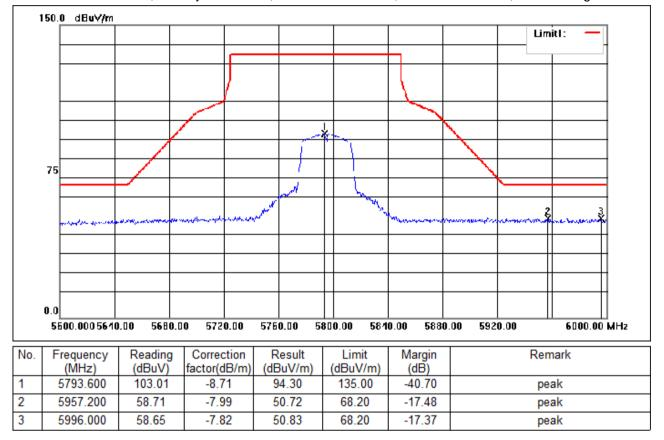
Test Mode: 06; Polarity: Horizontal; Modulation:802.11n; Bandwidth:40MHz; Channel:High
