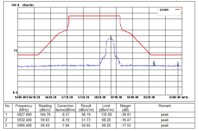
Test Mode: 06; Polarity: Horizontal; Modulation:802.11ac; Bandwidth:20MHz; Channel:High
