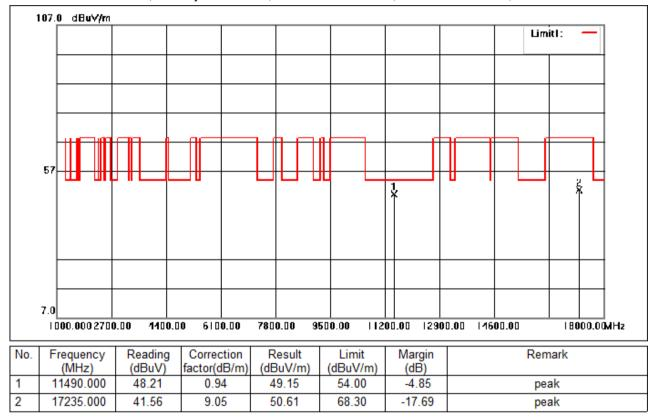
Test Mode: 06; Polarity: Horizontal; Modulation:802.11a; Bandwidth:20MHz; Channel:Low
