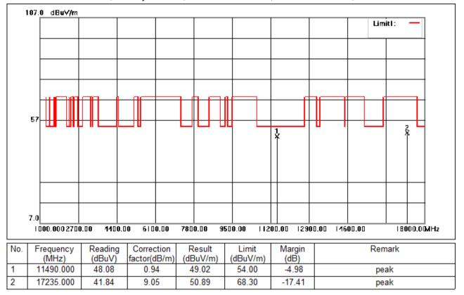
Test Mode: 06; Polarity: Vertical; Modulation:802.11a; Bandwidth:20MHz; Channel:Low
