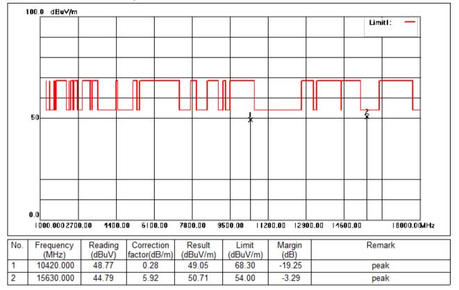
Test Mode: 05; Polarity: Vertical; Modulation:802.11ac; Bandwidth:80MHz; Channel:middle
