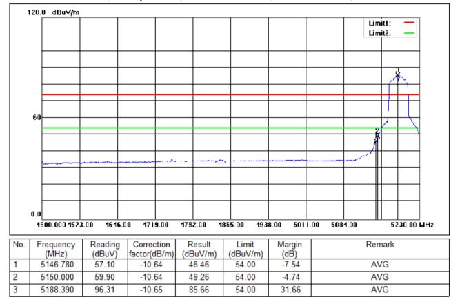
Test Mode: 05; Polarity: Vertical; Modulation:802.11ac; Bandwidth:40MHz; Channel:Low
