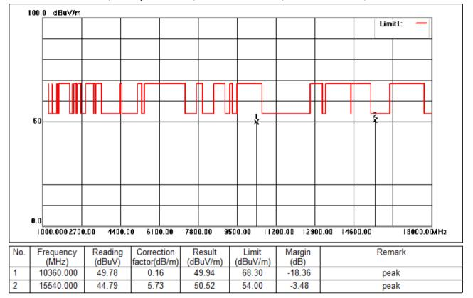
Test Mode: 05; Polarity: Horizontal; Modulation:802.11a; Bandwidth:20MHz; Channel:Low
