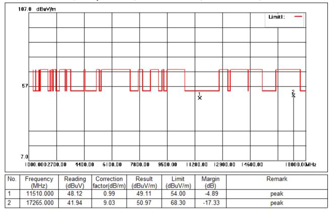
Test Mode: 06; Polarity: Horizontal; Modulation:802.11ac; Bandwidth:40MHz; Channel:Low
