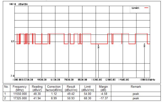
Test Mode: 06; Polarity: Horizontal; Modulation:802.11ac; Bandwidth:80MHz; Channel:middle
