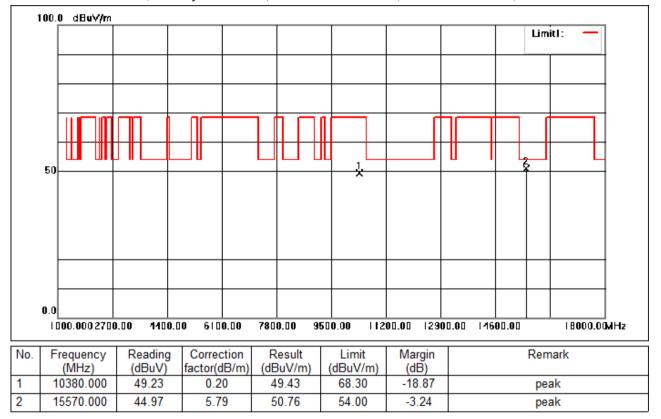
Test Mode: 05; Polarity: Horizontal; Modulation:802.11ac; Bandwidth:40MHz; Channel:Low
