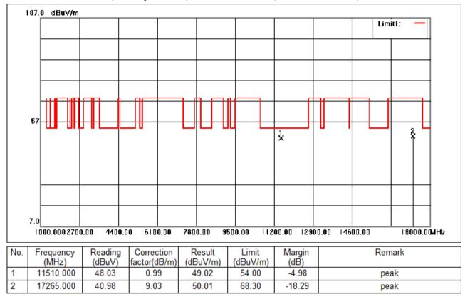
Test Mode: 06; Polarity: Vertical; Modulation:802.11n; Bandwidth:40MHz; Channel:Low
