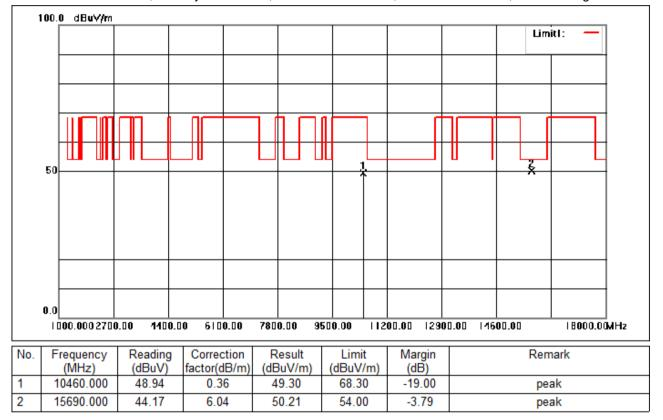
Test Mode: 05; Polarity: Horizontal; Modulation:802.11n; Bandwidth:40MHz; Channel:High
