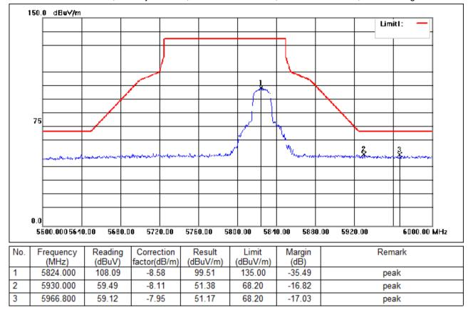
Test Mode: 06; Polarity: Vertical; Modulation:802.11n; Bandwidth:20MHz; Channel:High
