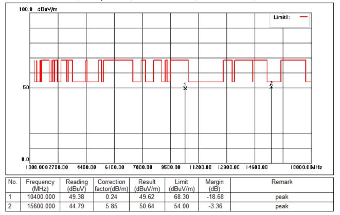
Test Mode: 05; Polarity: Vertical; Modulation:802.11a; Bandwidth:20MHz; Channel:middle
