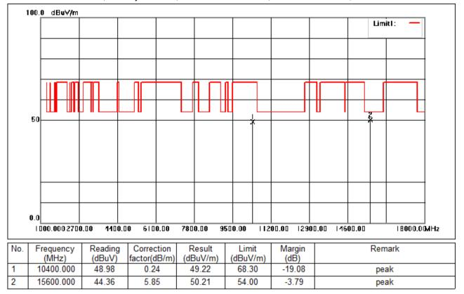
Test Mode: 05; Polarity: Vertical; Modulation:802.11ac; Bandwidth:20MHz; Channel:middle
