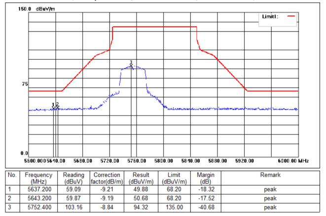
Test Mode: 06; Polarity: Horizontal; Modulation:802.11ac; Bandwidth:40MHz; Channel:Low
