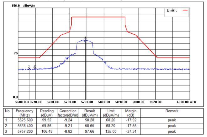
Test Mode: 06; Polarity: Vertical; Modulation:802.11n; Bandwidth:40MHz; Channel:Low
