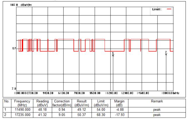
Test Mode: 06; Polarity: Horizontal; Modulation:802.11ac; Bandwidth:20MHz; Channel:Low
