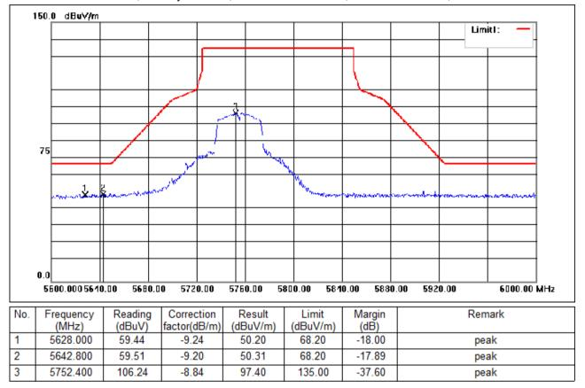
Test Mode: 06; Polarity: Vertical; Modulation:802.11ac; Bandwidth:40MHz; Channel:Low
