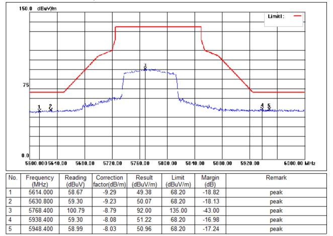
Test Mode: 06; Polarity: Horizontal; Modulation:802.11ac; Bandwidth:80MHz; Channel:middle
