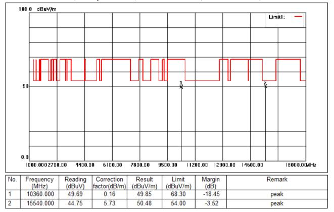
Test Mode: 05; Polarity: Horizontal; Modulation:802.11ac; Bandwidth:20MHz; Channel:Low
