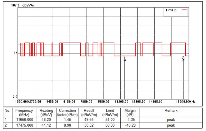
Test Mode: 06; Polarity: Vertical; Modulation:802.11ac; Bandwidth:20MHz; Channel:High
