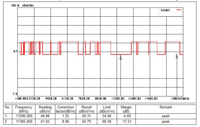
Test Mode: 06; Polarity: Horizontal; Modulation:802.11n; Bandwidth:40MHz; Channel:High
