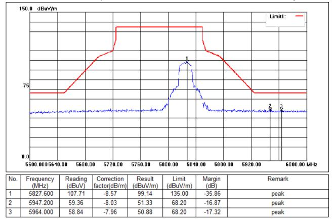
Test Mode: 06; Polarity: Vertical; Modulation:802.11ac; Bandwidth:20MHz; Channel:High
