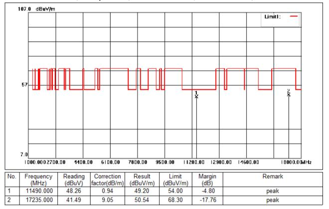
Test Mode: 06; Polarity: Vertical; Modulation:802.11ac; Bandwidth:20MHz; Channel:Low
