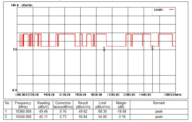
Test Mode: 05; Polarity: Vertical; Modulation:802.11n; Bandwidth:20MHz; Channel:Low
