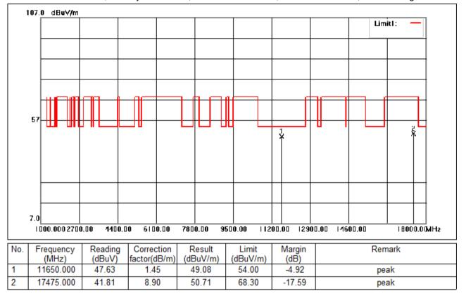
Test Mode: 06; Polarity: Horizontal; Modulation:802.11a; Bandwidth:20MHz; Channel:High
