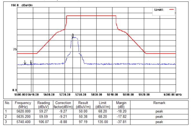
Test Mode: 06; Polarity: Horizontal; Modulation:802.11a; Bandwidth:20MHz; Channel:Low
