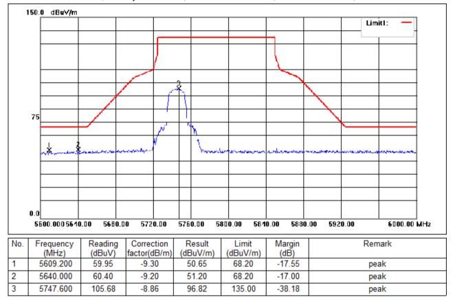
Test Mode: 06; Polarity: Horizontal; Modulation:802.11ac; Bandwidth:20MHz; Channel:Low
