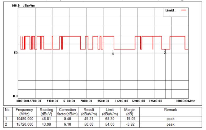
Test Mode: 05; Polarity: Horizontal; Modulation:802.11a; Bandwidth:20MHz; Channel:High
