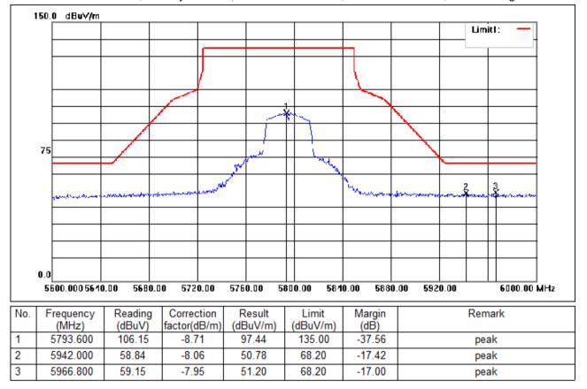
Test Mode: 06; Polarity: Vertical; Modulation:802.11n; Bandwidth:40MHz; Channel:High
