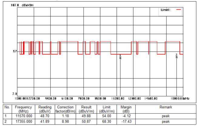
Test Mode: 06; Polarity: Horizontal; Modulation:802.11n; Bandwidth:20MHz; Channel:middle
