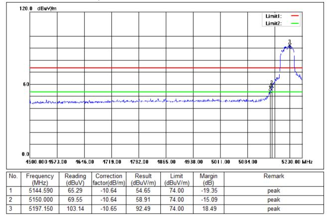
Test Mode: 05; Polarity: Horizontal; Modulation:802.11n; Bandwidth:40MHz; Channel:Low
