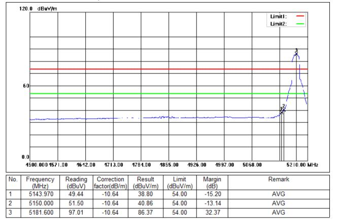
Test Mode: 05; Polarity: Horizontal; Modulation:802.11ac; Bandwidth:20MHz; Channel:Low
