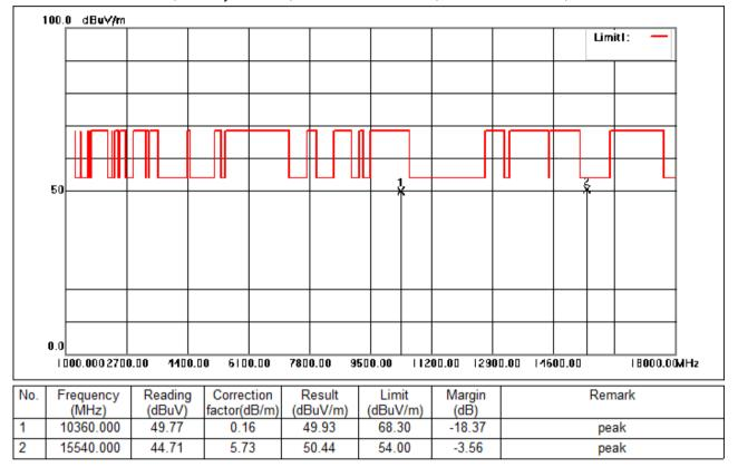
Test Mode: 05; Polarity: Vertical; Modulation:802.11ac; Bandwidth:20MHz; Channel:Low
