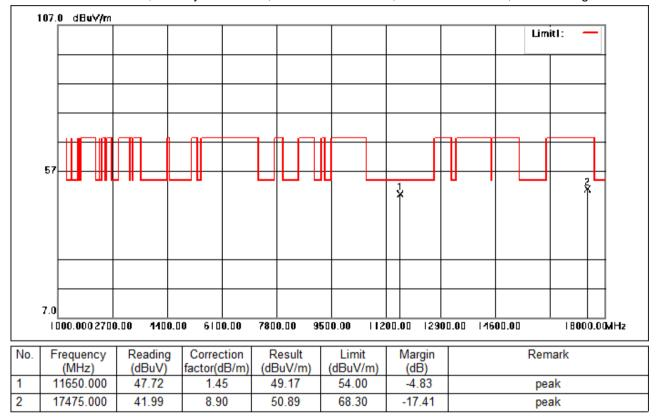
Test Mode: 06; Polarity: Horizontal; Modulation:802.11n; Bandwidth:20MHz; Channel:High
