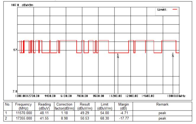
Test Mode: 06; Polarity: Horizontal; Modulation:802.11ac; Bandwidth:20MHz; Channel:middle
