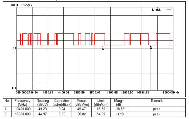
Test Mode: 05; Polarity: Vertical; Modulation:802.11n; Bandwidth:20MHz; Channel:middle
