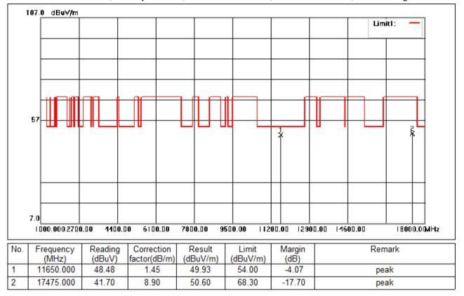
Test Mode: 06; Polarity: Vertical; Modulation:802.11n; Bandwidth:20MHz; Channel:High
