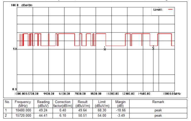
Test Mode: 05; Polarity: Vertical; Modulation:802.11n; Bandwidth:20MHz; Channel:High
