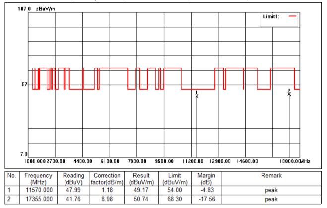
Test Mode: 06; Polarity: Vertical; Modulation:802.11ac; Bandwidth:20MHz; Channel:middle
