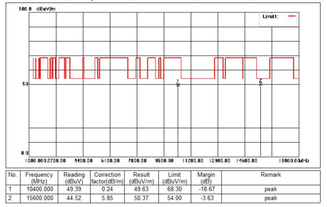
Test Mode: 05; Polarity: Horizontal; Modulation:802.11ac; Bandwidth:20MHz; Channel:middle
