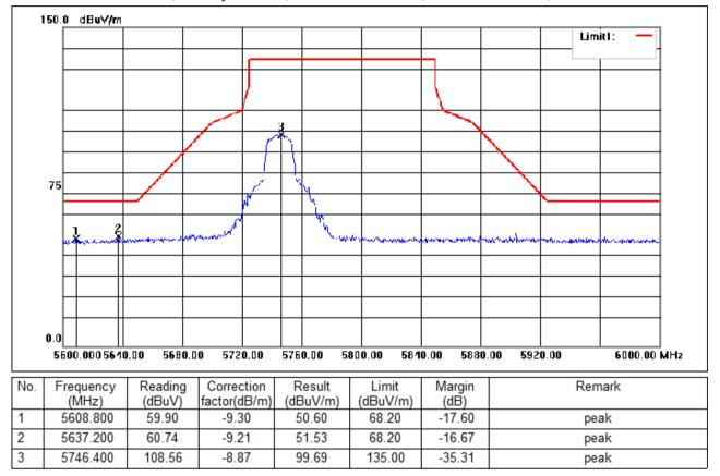
Test Mode: 06; Polarity: Vertical; Modulation:802.11n; Bandwidth:20MHz; Channel:Low
