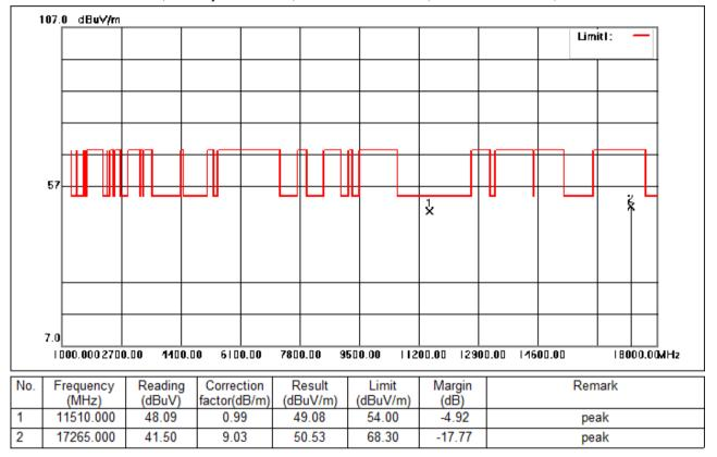
Test Mode: 06; Polarity: Horizontal; Modulation:802.11n; Bandwidth:40MHz; Channel:Low
