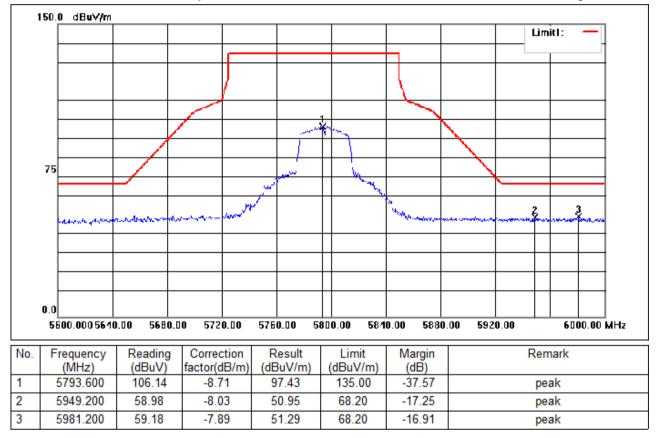
Test Mode: 06; Polarity: Vertical; Modulation:802.11ac; Bandwidth:40MHz; Channel:High
