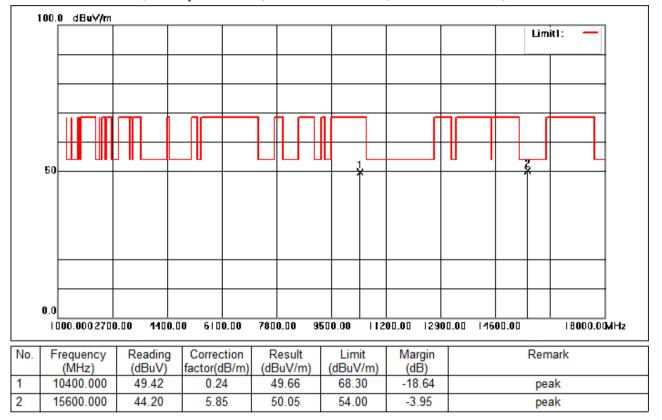
Test Mode: 05; Polarity: Horizontal; Modulation:802.11n; Bandwidth:20MHz; Channel:middle
