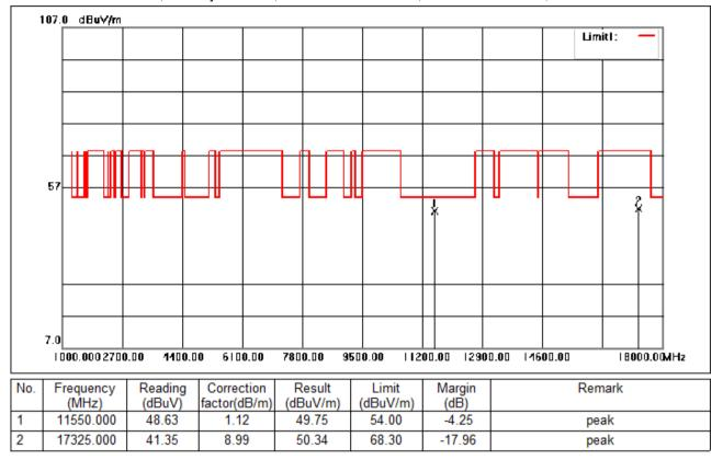
Test Mode: 06; Polarity: Vertical; Modulation:802.11ac; Bandwidth:80MHz; Channel:middle
