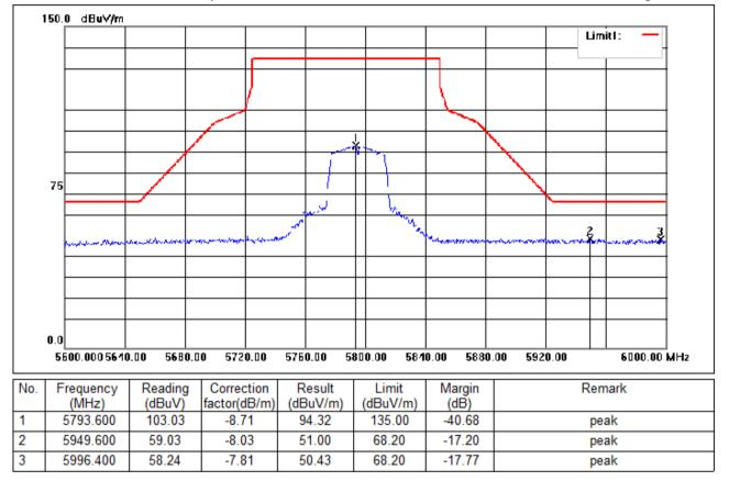
Test Mode: 06; Polarity: Horizontal; Modulation:802.11ac; Bandwidth:40MHz; Channel:High
