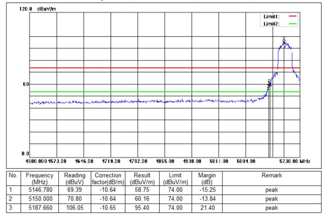
Test Mode: 05; Polarity: Vertical; Modulation:802.11n; Bandwidth:40MHz; Channel:Low
