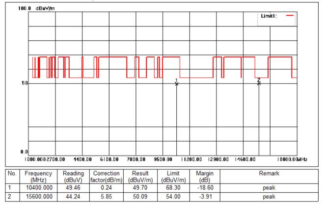
Test Mode: 05; Polarity: Horizontal; Modulation:802.11a; Bandwidth:20MHz; Channel:middle
