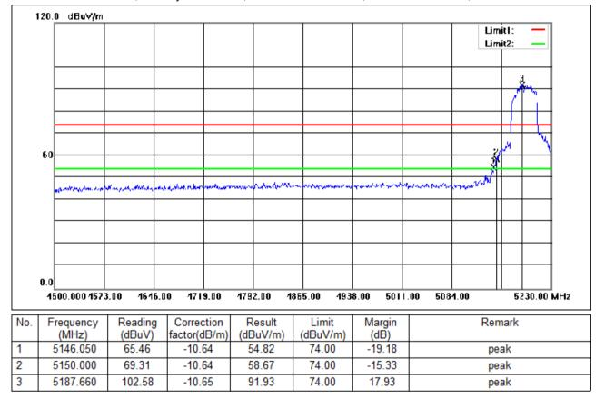
Test Mode: 05; Polarity: Horizontal; Modulation:802.11ac; Bandwidth:40MHz; Channel:Low
