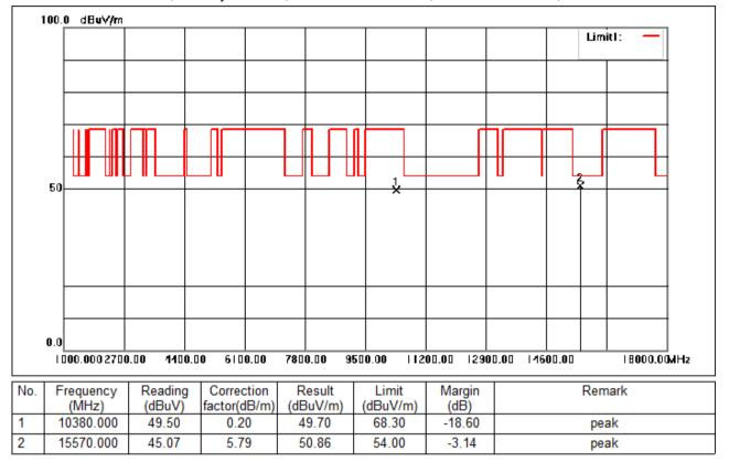
Test Mode: 05; Polarity: Vertical; Modulation:802.11ac; Bandwidth:40MHz; Channel:Low
