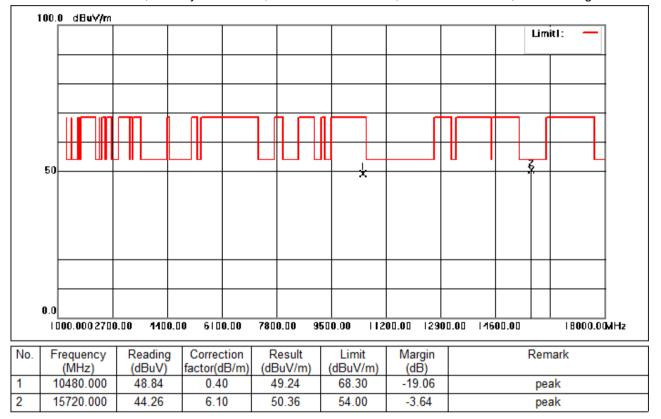
Test Mode: 05; Polarity: Horizontal; Modulation:802.11ac; Bandwidth:20MHz; Channel:High
