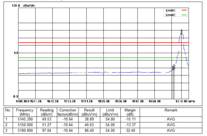
Test Mode: 05; Polarity: Horizontal; Modulation:802.11a; Bandwidth:20MHz; Channel:Low
