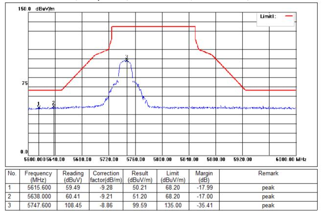
Test Mode: 06; Polarity: Vertical; Modulation:802.11ac; Bandwidth:20MHz; Channel:Low
