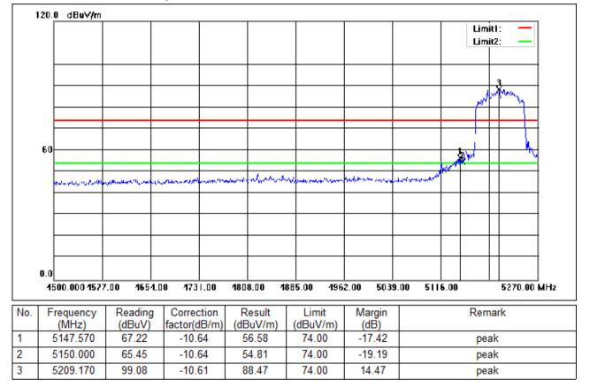
Test Mode: 05; Polarity: Horizontal; Modulation:802.11ac; Bandwidth:80MHz; Channel:middle
