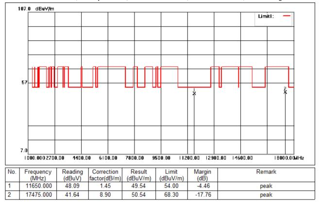
Test Mode: 06; Polarity: Vertical; Modulation:802.11a; Bandwidth:20MHz; Channel:High
