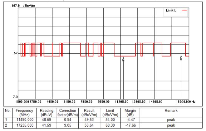
Test Mode: 06; Polarity: Vertical; Modulation:802.11n; Bandwidth:20MHz; Channel:Low
