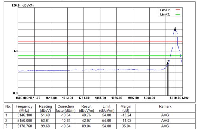
Test Mode: 05; Polarity: Vertical; Modulation:802.11n; Bandwidth:20MHz; Channel:Low
