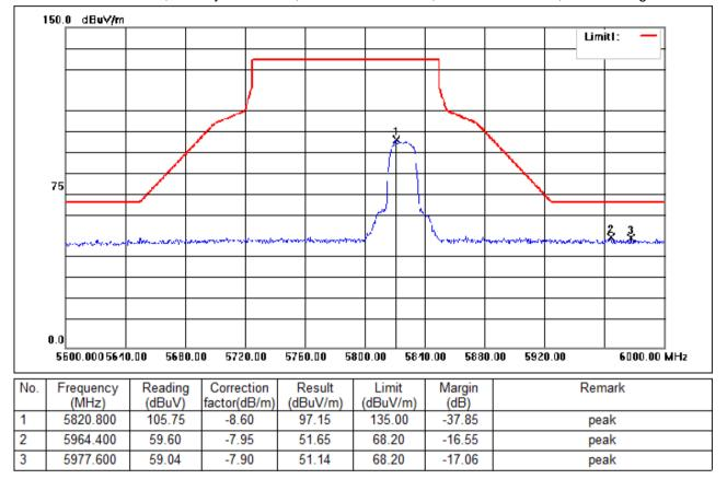
Test Mode: 06; Polarity: Horizontal; Modulation:802.11a; Bandwidth:20MHz; Channel:High
