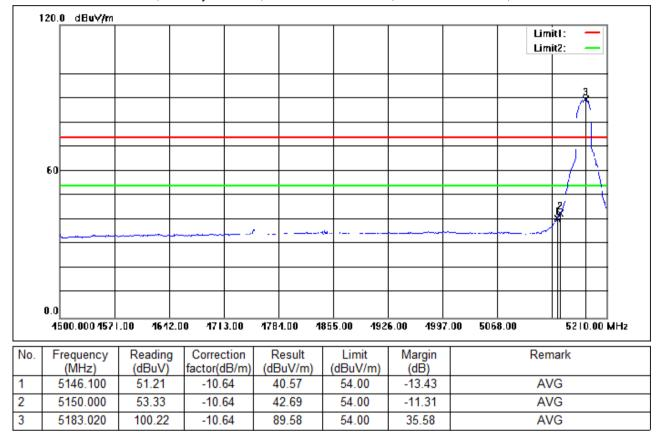
Test Mode: 05; Polarity: Vertical; Modulation:802.11ac; Bandwidth:20MHz; Channel:Low
