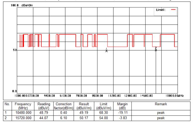
Test Mode: 05; Polarity: Vertical; Modulation:802.11ac; Bandwidth:20MHz; Channel:High
