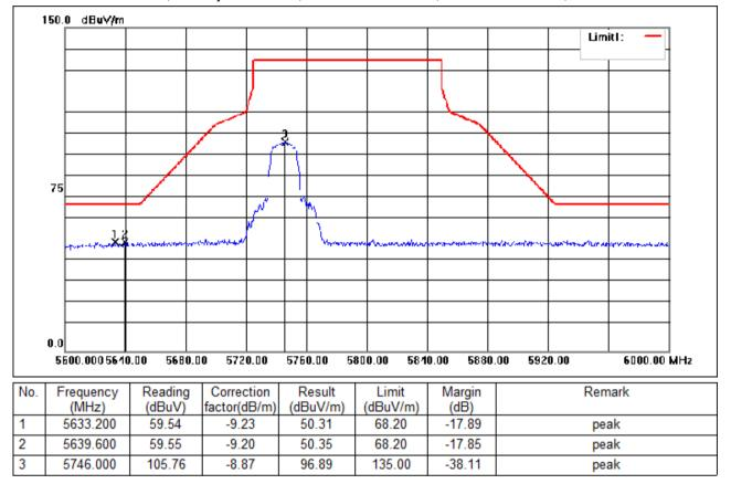
Test Mode: 06; Polarity: Horizontal; Modulation:802.11n; Bandwidth:20MHz; Channel:Low
