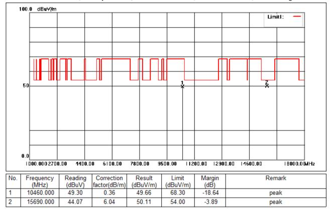
Test Mode: 05; Polarity: Vertical; Modulation:802.11n; Bandwidth:40MHz; Channel:High
