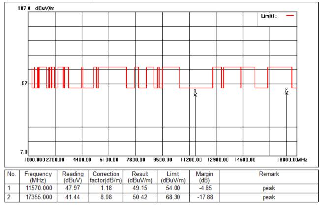
Test Mode: 06; Polarity: Horizontal; Modulation:802.11a; Bandwidth:20MHz; Channel:middle
