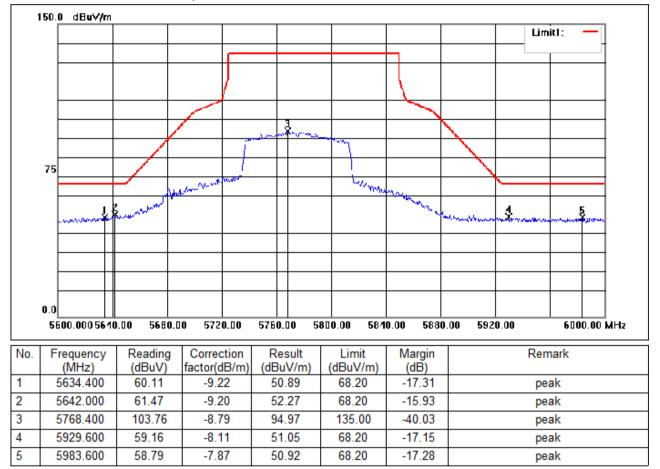
Test Mode: 06; Polarity: Vertical; Modulation:802.11ac; Bandwidth:80MHz; Channel:middle
