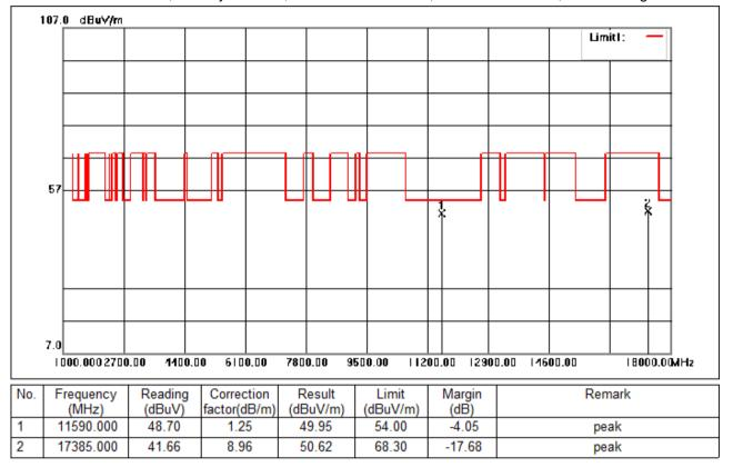
Test Mode: 06; Polarity: Vertical; Modulation:802.11ac; Bandwidth:40MHz; Channel:High
