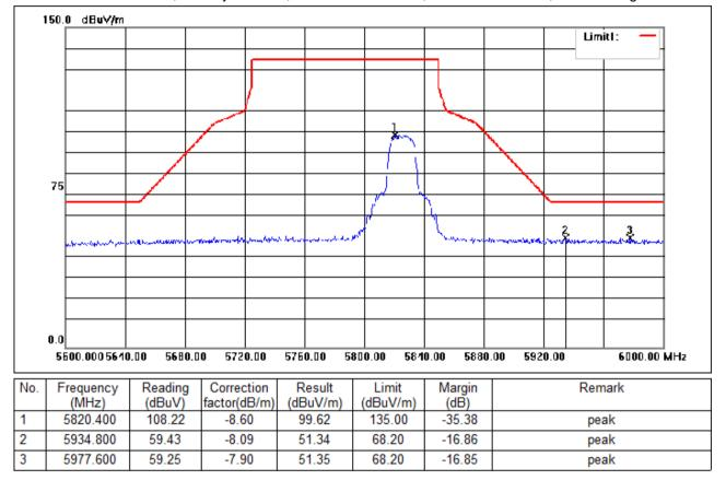
Test Mode: 06; Polarity: Vertical; Modulation:802.11a; Bandwidth:20MHz; Channel:High
