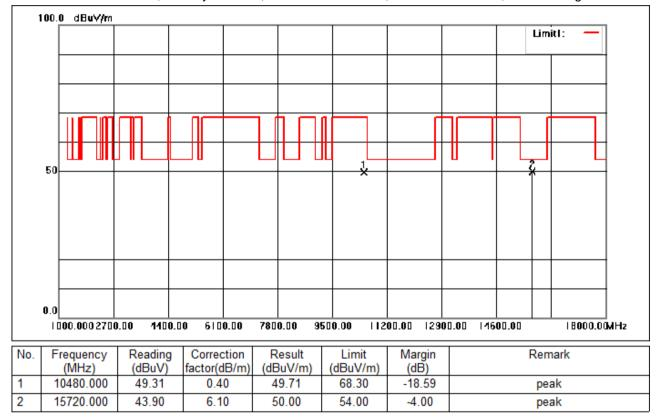
Test Mode: 05; Polarity: Vertical; Modulation:802.11a; Bandwidth:20MHz; Channel:High
