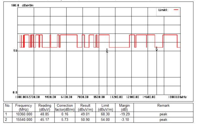
Test Mode: 05; Polarity: Vertical; Modulation:802.11a; Bandwidth:20MHz; Channel:Low
