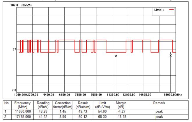
Test Mode: 06; Polarity: Horizontal; Modulation:802.11ac; Bandwidth:20MHz; Channel:High
