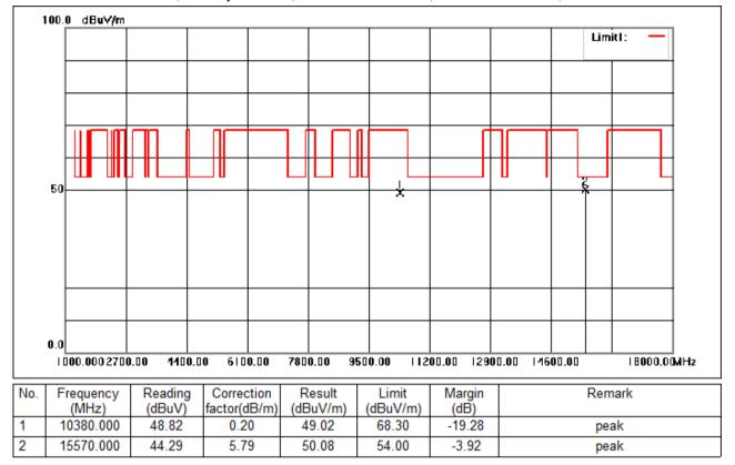
Test Mode: 05; Polarity: Vertical; Modulation:802.11n; Bandwidth:40MHz; Channel:Low
