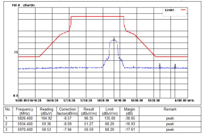
Test Mode: 06; Polarity: Horizontal; Modulation:802.11n; Bandwidth:20MHz; Channel:High
