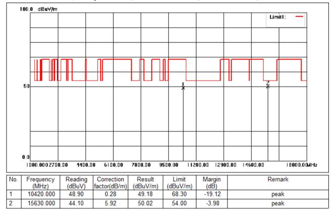
Test Mode: 05; Polarity: Horizontal; Modulation:802.11ac; Bandwidth:80MHz; Channel:middle
