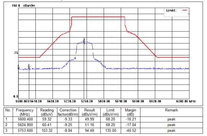
Test Mode: 06; Polarity: Horizontal; Modulation:802.11n; Bandwidth:40MHz; Channel:Low
