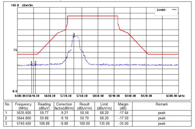
Test Mode: 06; Polarity: Vertical; Modulation:802.11a; Bandwidth:20MHz; Channel:Low
