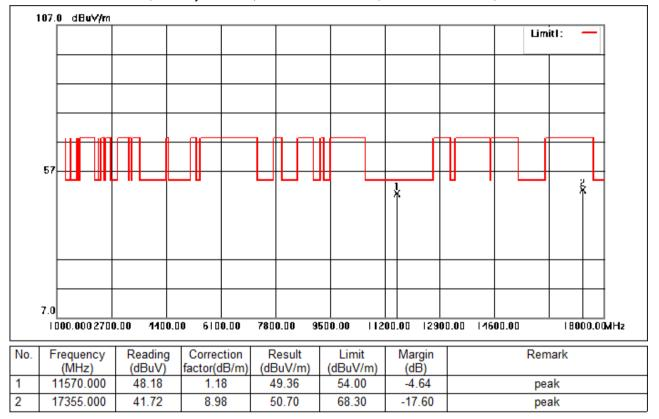
Test Mode: 06; Polarity: Vertical; Modulation:802.11n; Bandwidth:20MHz; Channel:middle
