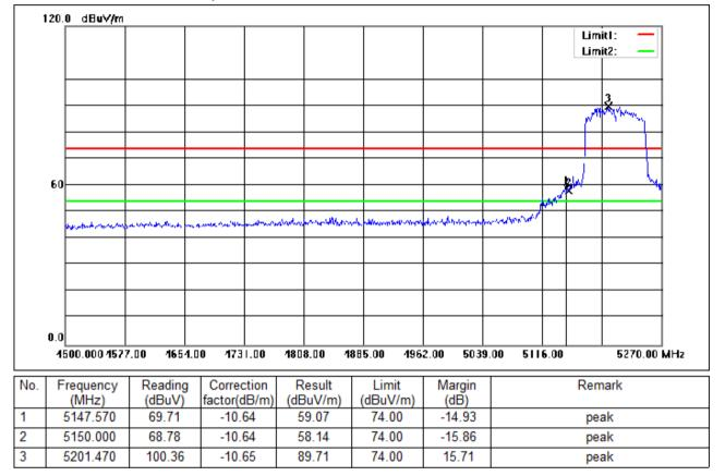
Test Mode: 05; Polarity: Vertical; Modulation:802.11ac; Bandwidth:80MHz; Channel:middle
