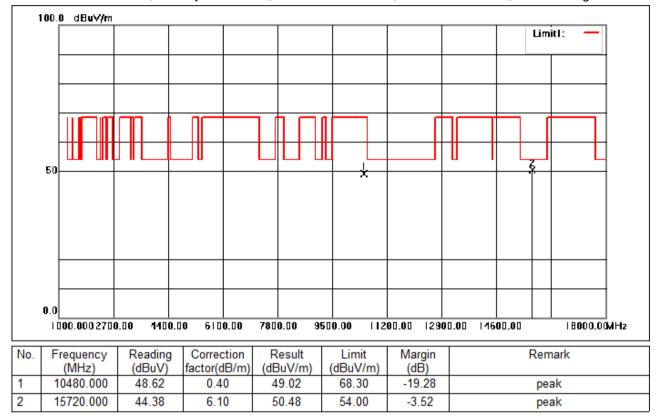
Test Mode: 05; Polarity: Horizontal; Modulation:802.11n; Bandwidth:20MHz; Channel:High
