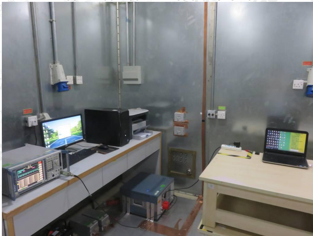
FCC RADIATED EMISSION TEST SETUP
