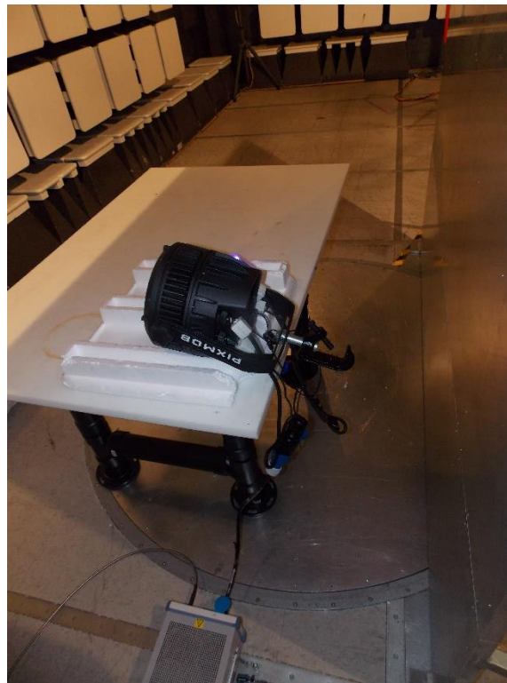
Figure 8.2-4: Conducted emissions – from AC mains power ports setup photo
