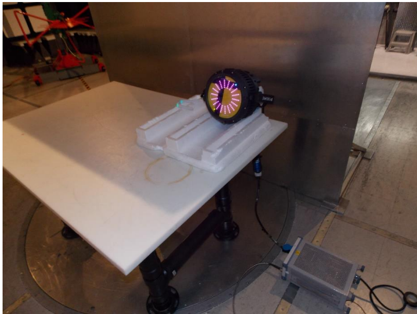
Figure 8.2-3: Conducted emissions – from AC mains power ports setup photo
