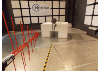
Figure 8.1-3: Radiated emissions setup photo - below 1 GHz
